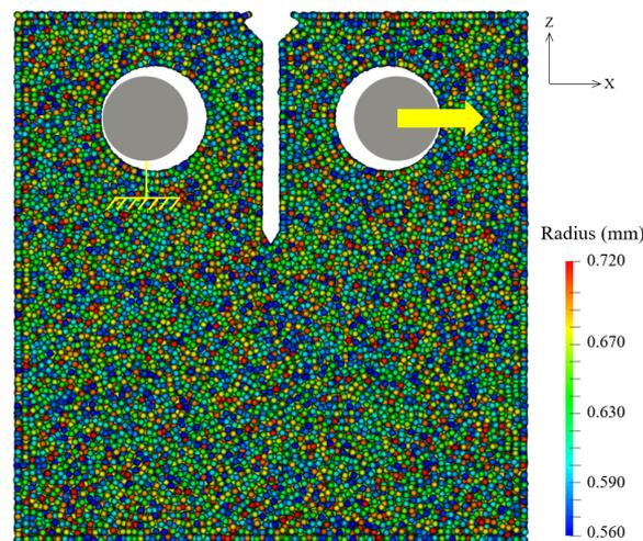
**Figure 7.** Distribution of the discrete elements radius in a full MS CT specimen. The discrete elements have an average radius of 640  $\mu\text{m}$ . Rigid pins are in both holes of the CT specimen.
