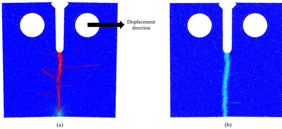
**Figure 11.** Crack propagation in the full MS CT specimen (a) and in the full MS-TiC CT specimen (b).
