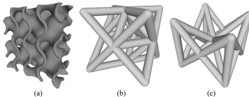
**Figure 1.** Topological cell of reinforcement—gyroid (a), octet-truss (b) and FBCCZ (c).
