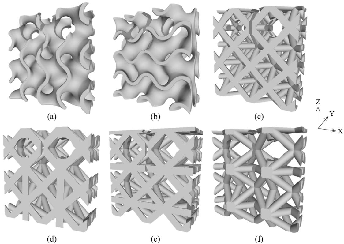
**Figure 4.** Topological inserts cut according to a CT specimen—Z-orientation gyroid (Gyroid\_01) (a), X-orientation gyroid (Gyroid\_02) (b), octet-truss (c), Z-orientation FBCCZ (FBCCZ\_01) (d), X-orientation FBCCZ (FBCCZ\_02) (e) and Y-orientation FBCCZ (FBCCZ\_03) (f).
