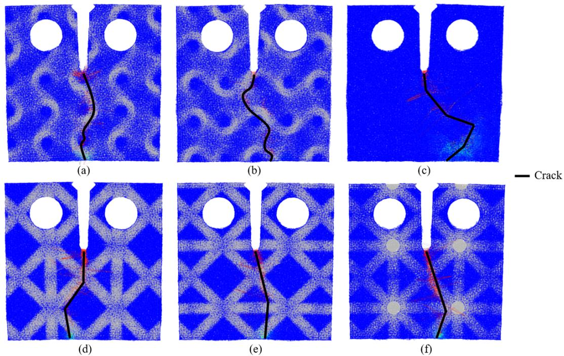
**Figure 13.** Crack paths in the metal which surrounds the MS-TiC topologies (MS) according to the failure stress of the DEM bonds. The red color of the bonds corresponds to the MS failure stress. Gyroid\_01 (a), Gyroid\_02 (b), octet-truss (c), FBCZZ\_01 (d), FBCCZ\_02 (e) and FBCCZ\_03 (f).
