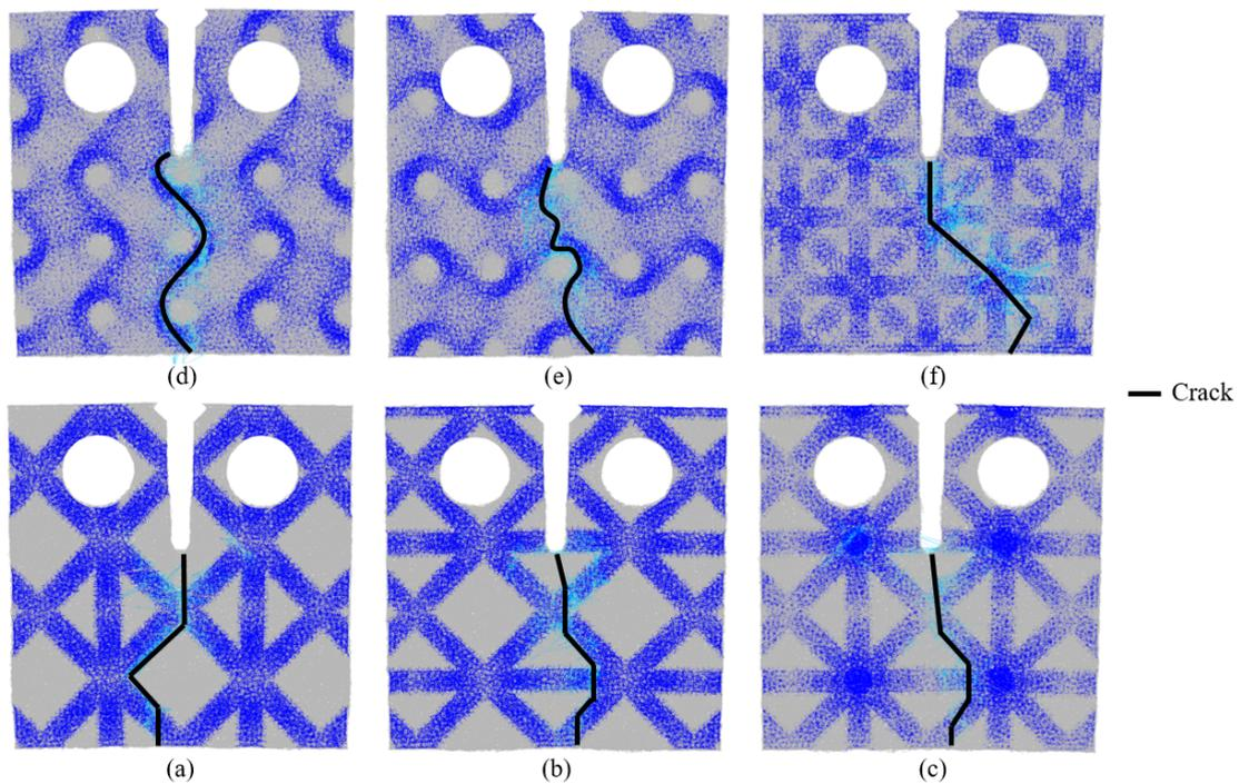
**Figure 12.** Crack paths in the MS-TiC inserts according to the failure stress of the DEM bonds. The blue color of the bonds corresponds to the MS-TiC failure stress. Gyroid\_01 (a), Gyroid\_02 (b), octet-truss (c), FBCZZ\_01 (d), FBCCZ\_02 (e) and FBCCZ\_03 (f).
