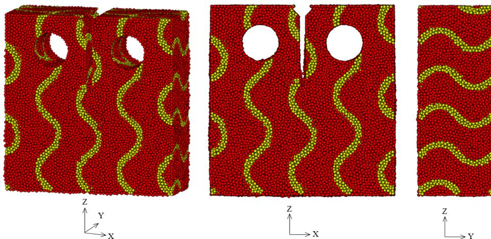
Figure 6. Views of the DEM domain of the Z-orientation gyroid (Gyroid\_01). The gyroid is represented by yellow discrete elements which correspond to the MS-TiC particles, whereas red elements correspond to the MS matrix.
