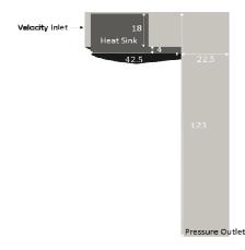
Fig. 2. Dimensions (in mm) of the domain.
