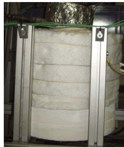
Fig. 3. Stirling engine heating system.
