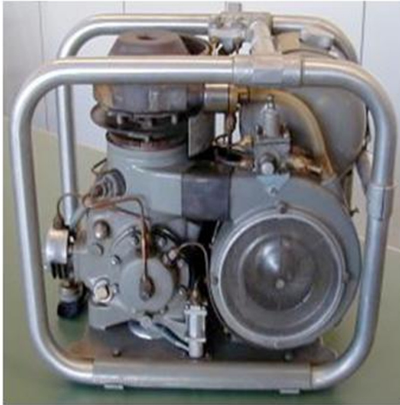
Fig. 16 250 We Philips Stirling Refrigerating Machine. Reproduced from WikiVisually. Available from: https://wikivisually.com/wiki/Stirling_heat_engine .
