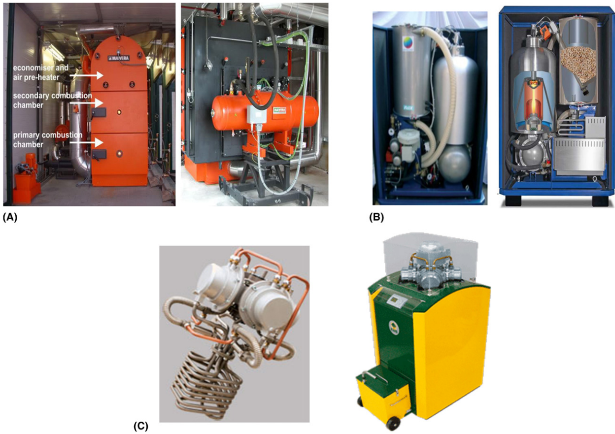
Fig. 13 Stirling engine cogeneration unit working with biomass. (A) Cogeneration unit “Stirling DK” ayant une puissance de 35 kW au Denmark (biomass, gasification) (Reproduced from Obernberger I, Carlsen H, Biedermann F. State-of-the art and future developments regarding small-scale biomass CHP systems with a special focus on ORC AND Stirling engine technologies. In: International Nordic bioenergy conference; 2003.). (B) Microcogeneration unit “Sunmachine” (biomass, pellets) (Reproduced from Crema L. et al. , Development of a pellet boiler with Stirling engine for m-CHP domestic application. Energy, Sustain Soc 2011;15.). (C) Wood Stirling micro CHP boiler (Reproduced from Stirlingpowermodule. Available from: www.stirlingpowermodule.com ).
