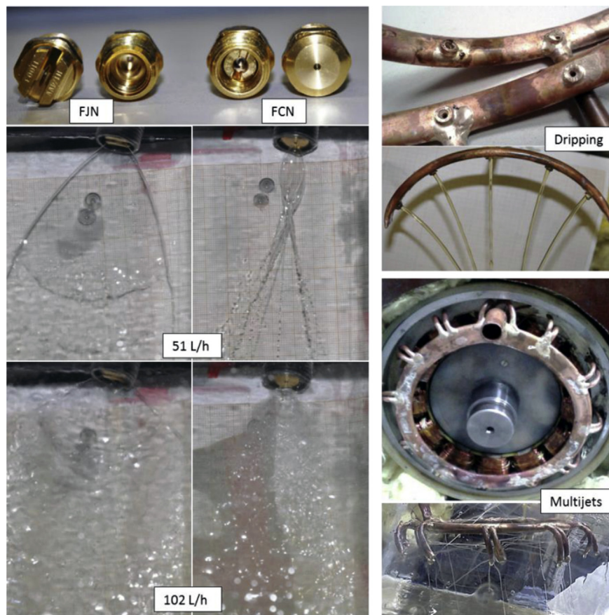
Fig. 5. Oil flow pattern for the flat jet nozzle (FJN) and the full cone nozzle (FCN) for low (top: 51 L/h) and high (bottom: 102 L/h) flow rates at 50 °C.
