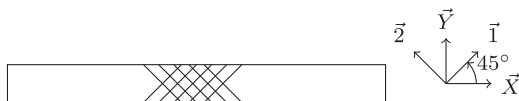
Fig. 10. Material coordinate system ( \vec{1}, \vec{2} ) according to the specimen coordinate system ( \vec{X}, \vec{Y} ) for in-plane shear tests.
