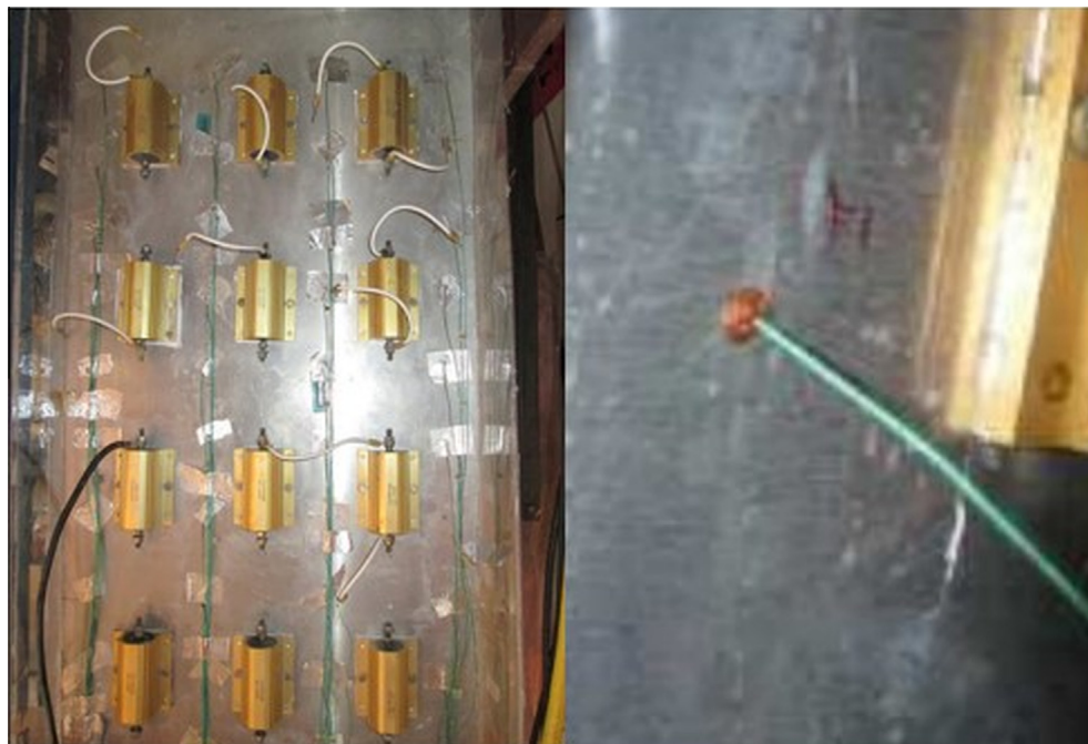
Fig. 5. The thermocouples in real site.
