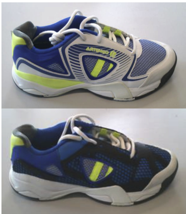
Fig. 1. Lateral view of the prototypes with flexible upper (up) and stiff upper (down).
