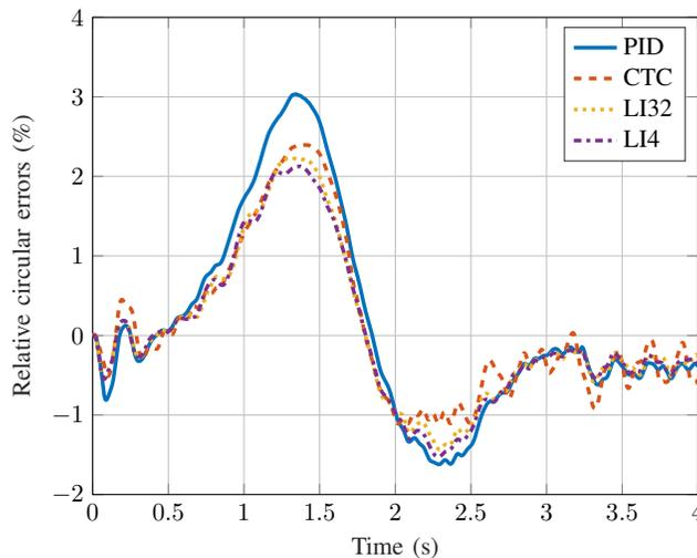
Fig. 2. Time history of the relative circularity errors  $\epsilon_c$  for the four compared controllers PID, CTC, LI32 and LI4.
