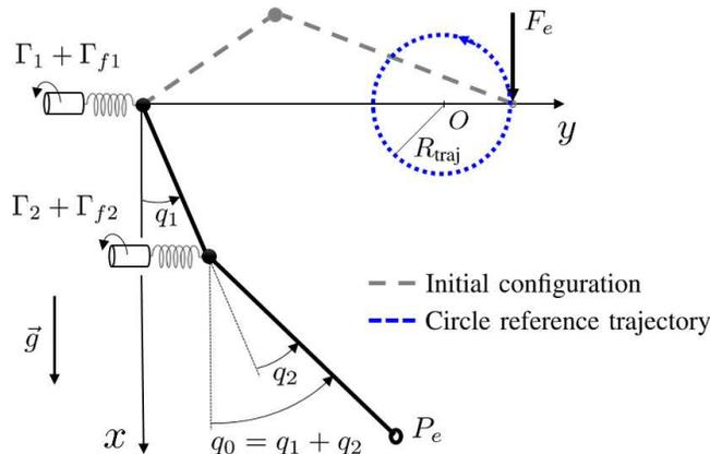
Fig. 1. Two degree-of-freedom benchmark manipulator.
