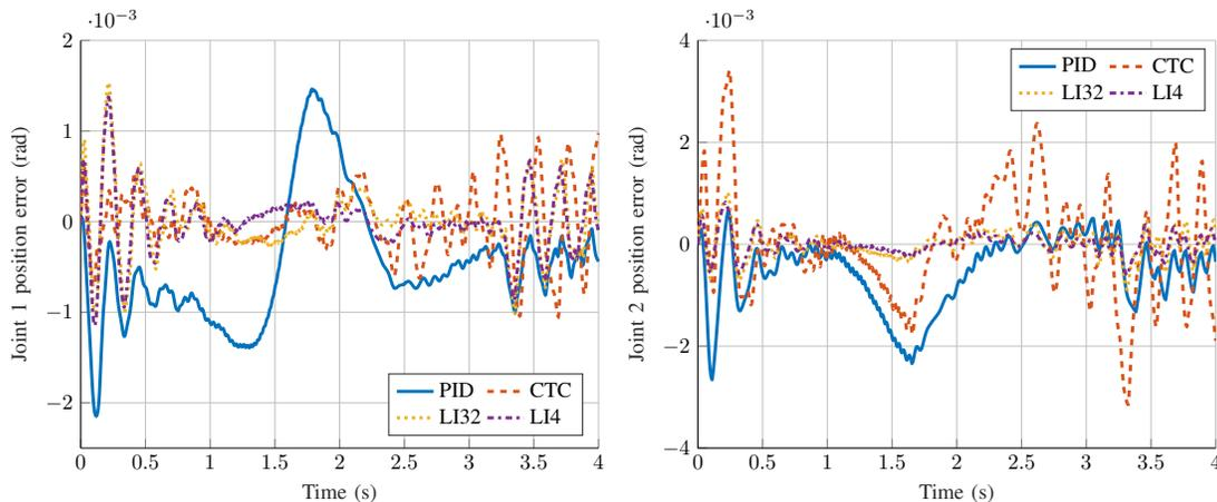
Fig. 3. Time history of the joint position errors.
