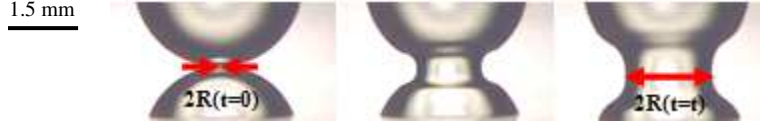
Figure 11: schematic of the evolution of the capillary liquid bridge during the coalescence of vertically aligned drops.
