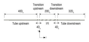
Fig.2: Sketch of the numerical test bench with  $P=10D_{h}$ .
