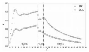
Fig.12: Evolution of the swirl number in the STE and ST3L and downstream at Re=10 000.
