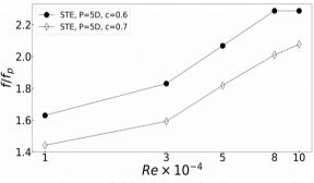
Fig.8: Evolution of  $f/f_p$  with Re for the STE with aspect ratio c=0.6 and c=0.7.
