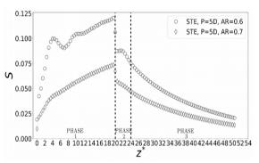
Fig.6: Evolution of the swirl number along the STE with c=0.6 and c=0.7 and downstream at Re=10 000.
