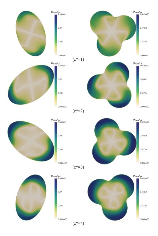
Fig.11: Axial evolution of the tangential velocity inside the first twist pitch of the STE (left) and ST3L (right).
