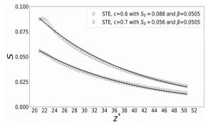
Fig.7: Evolution of the swirl intensity in STE with c=0.6 and c=0.7 and curve fitting.
