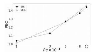
Fig.16: Evolution of the PEC for the STE and the ST3L with the Reynolds number.
