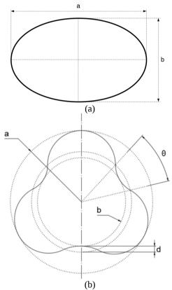
Fig.1: (a) sketch of an elliptic cross-section, (b) sketch of a three-lobed cross-section.
