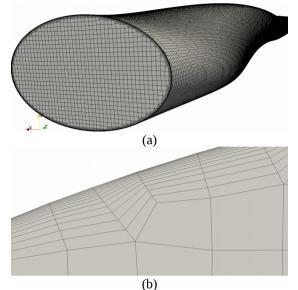
Fig.4: (a) Clip of the meshed geometry with mesh 2, (b) details of the mesh close to the wall of the tube.
