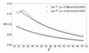
Fig. 13. Evolution of the swirl intensity downstream the STE and ST3L and curve fitting at Re=10 000.
