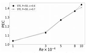
Fig.10: Evolution of the PEC with Re for the STE with aspect ratio c=0.6 and c=0.7
