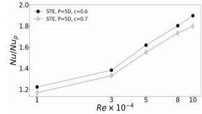
Fig.9: Evolution of  $Nu/Nu_p$  with Re for the STE with aspect ratio c=0.6 and c=0.7.
