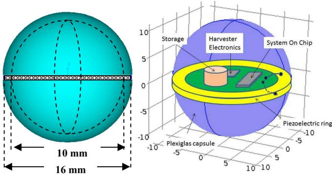
Figure 1: Illustration of the spherical resonator
