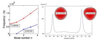
Figure 2: Natural frequencies of tortionless modes for the composite sensor
