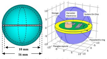
Figure 1: Illustration of the spherical resonator
