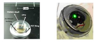
Figure 3: The autonomous acoustic sensor with the embedded electronics
