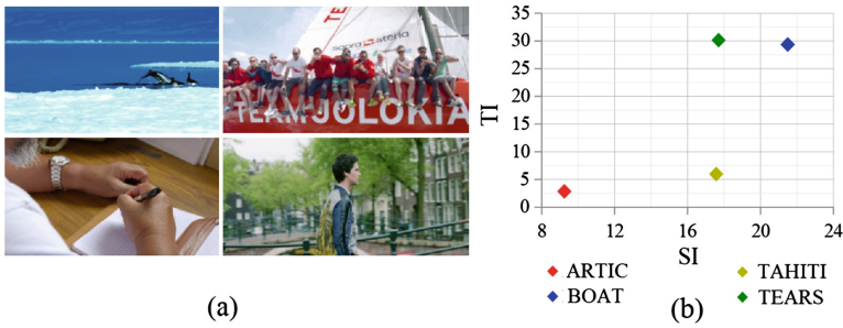
Fig. 3. (a) Test video sequences used in the experiments, clockwise from top left: Artic, Boat, Tears, Tahiti. (b) SI TI index.
