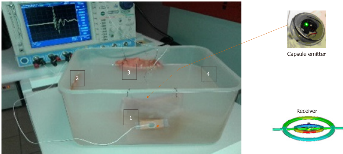
Figure 10 Illustration of the measurement cell showing the spatial distribution of the emitter capsule embedded in the volume of agar at controlled distance of the different bio-tissue samples equipped with micro-resonators receivers.
