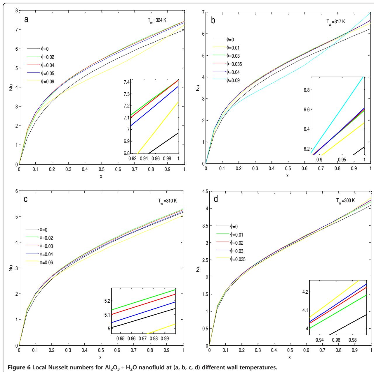
**Figure 6** Local Nusselt numbers for  $\text{Al}_2\text{O}_3 + \text{H}_2\text{O}$  nanofluid at (a, b, c, d) different wall temperatures.
