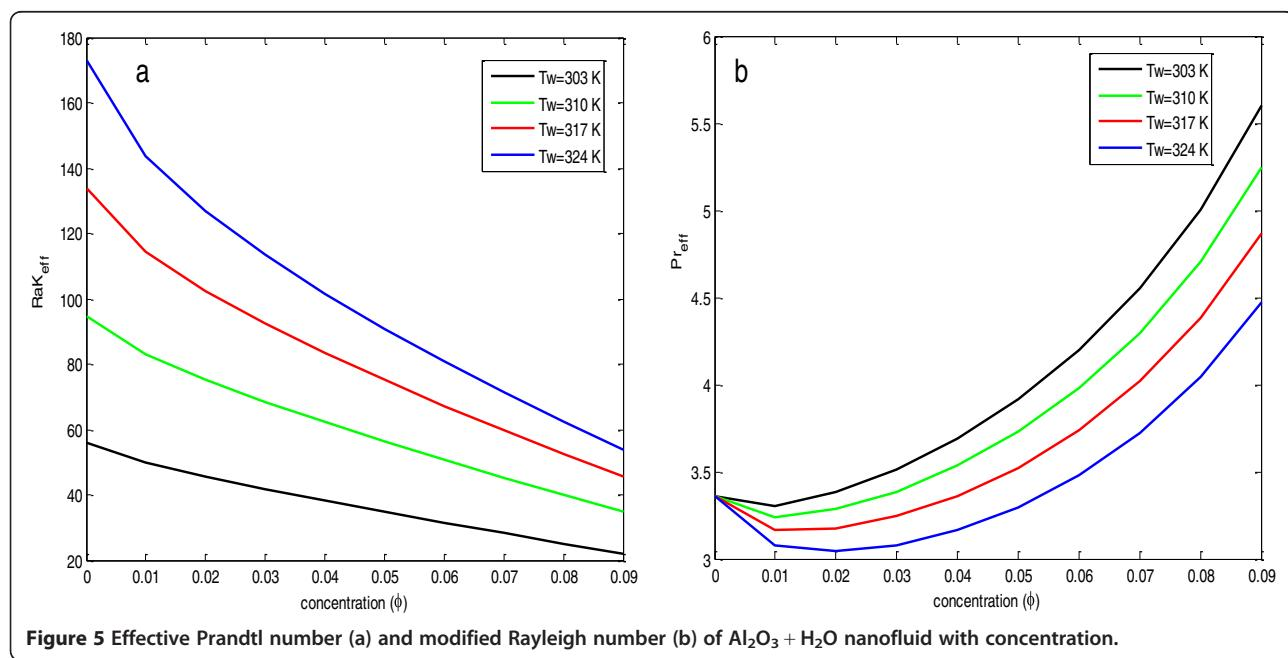
Figure 5 Effective Prandtl number (a) and modified Rayleigh number (b) of  $\text{Al}_2\text{O}_3 + \text{H}_2\text{O}$  nanofluid with concentration.
