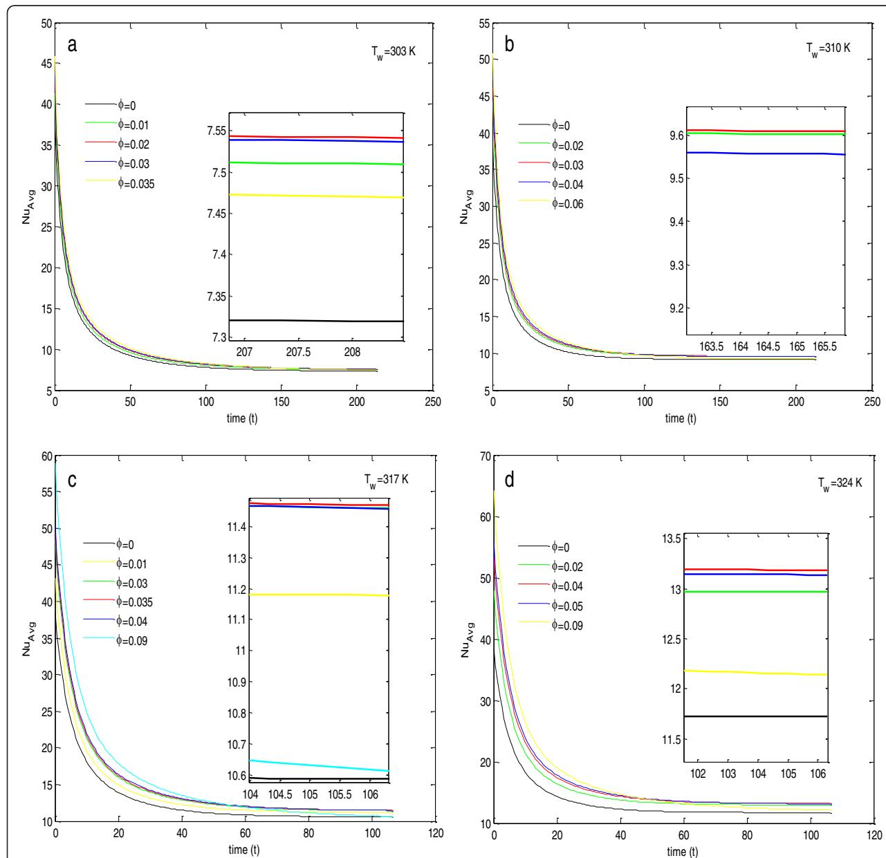
**Figure 4** Average Nusselt numbers for  $\text{Al}_2\text{O}_3 + \text{H}_2\text{O}$  nanofluid at (a, b, c, d) different wall temperatures.
