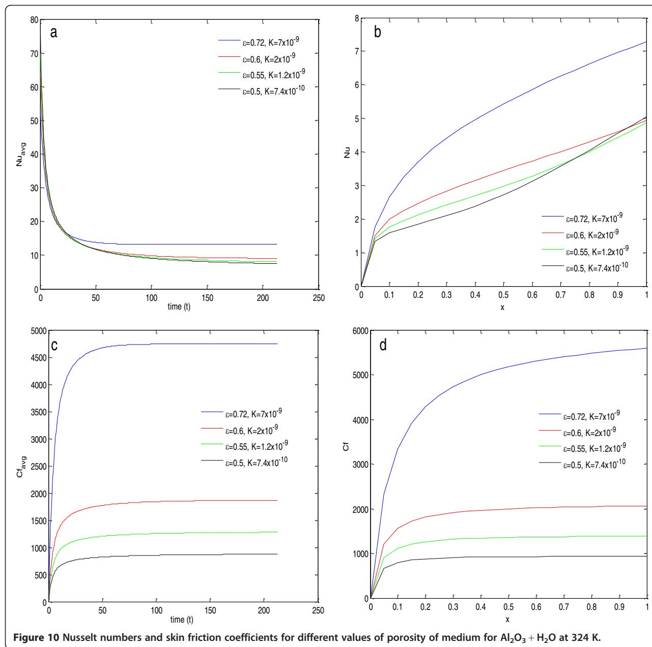
**Figure 10** Nusselt numbers and skin friction coefficients for different values of porosity of medium for  $\text{Al}_2\text{O}_3 + \text{H}_2\text{O}$  at 324 K.
