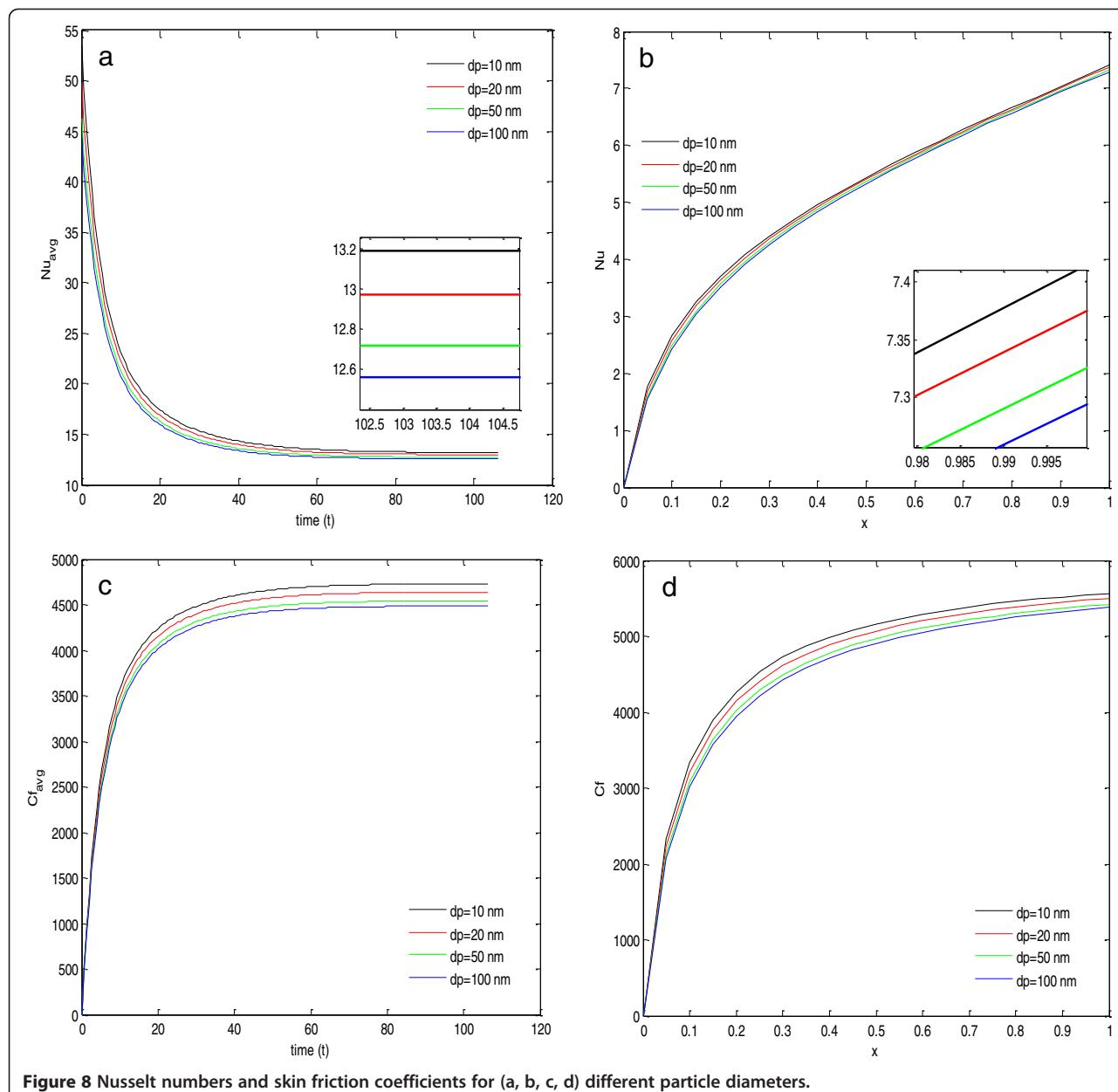
**Figure 8** Nusselt numbers and skin friction coefficients for (a, b, c, d) different particle diameters.
