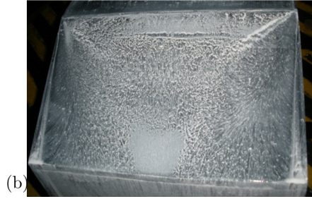
Fig. 5. (a) Drag coefficient versus the Reynolds number and (b) the baseline flow visualization performed in the present study for Re_L = 2.08 \times 10^6 .
