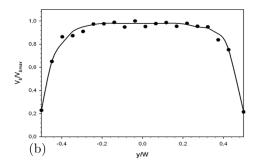
Fig. 4. Actuator flow characterization: (a) velocity measurement set-up and (b) typical blowing velocity profile along the slot length (W).
