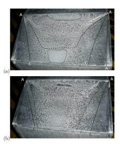
Fig. 8. Cartography of the friction lines on the rear window ( $Re_L = 2.08 \times 10^6$ ,  $V_0 = 30$  m/s,  $V_b = 16.5$  m/s), (a): without control and (b) with control
