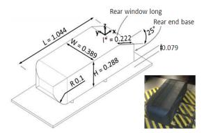
Fig. 2. Geometry of the Ahmed car model (dimensions in m), Ahmed *et al.* (Ahmed, Ramm, and Faltin 1984).
