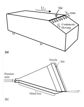
Fig. 3. Description of the control device: (a) overview and (b) design of blowing actuator nozzle.
