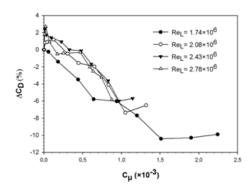
Fig. 6. Drag reduction as function of the steady momentum coefficient for different  $Re_L$ .
