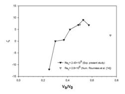
Fig. 7. Actuator efficiency versus the blowing velocity: comparison between the present experimental results and the numerical results of Rouméas *et al.* (Rouméas, Gilliéron, and Kourta 2009).
