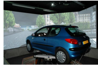
Fig. 8. SHERPA driving simulator.
