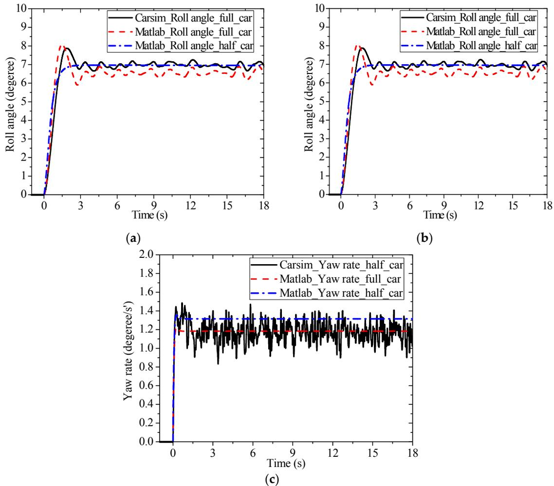
Figure 10. Results with road Level ISO-A excitation (steering wheel angle was 10° at 80 km/h). (a) Roll angle; (b) Roll rate; (c) Yaw rate.
