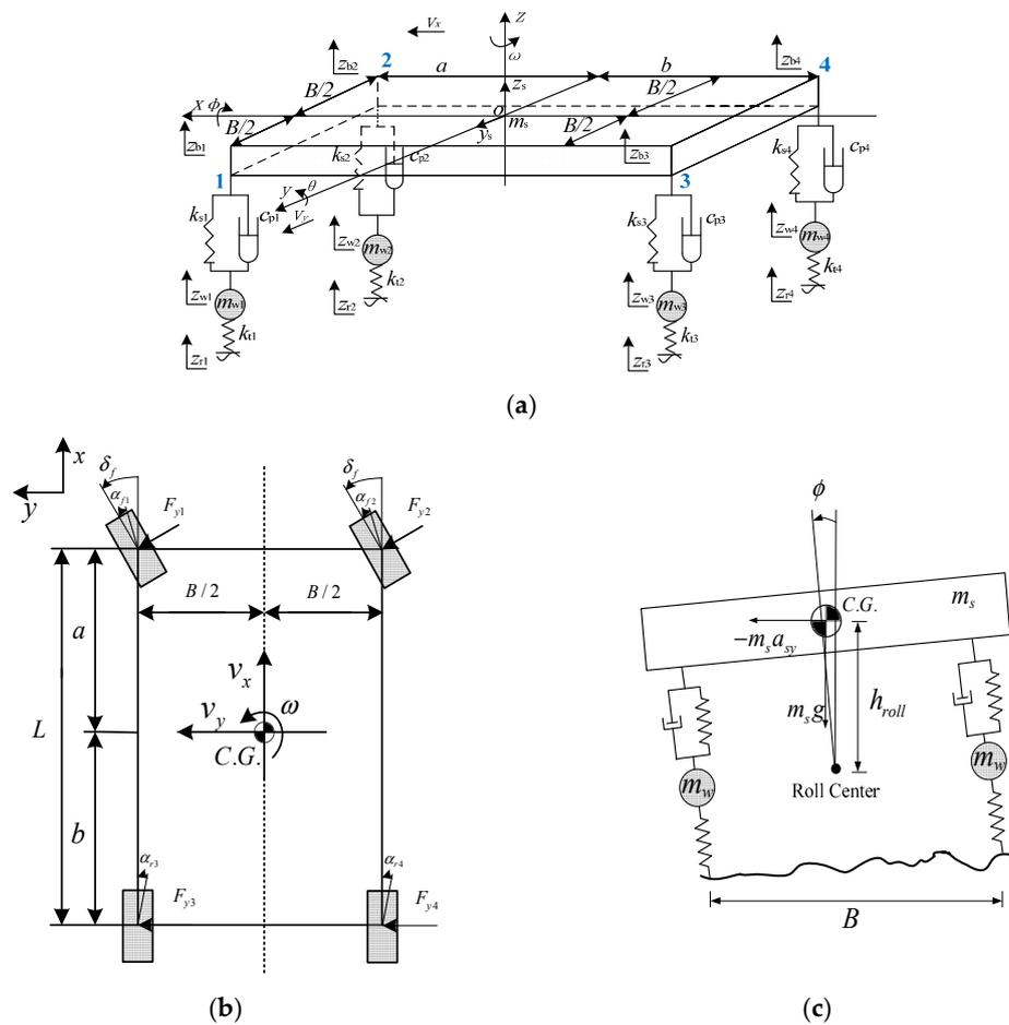
**Figure 7.** 9-DOF vehicle dynamics model. (a) Full-car dynamics model. (b) Lateral dynamics model. (c) Roll dynamics model.
