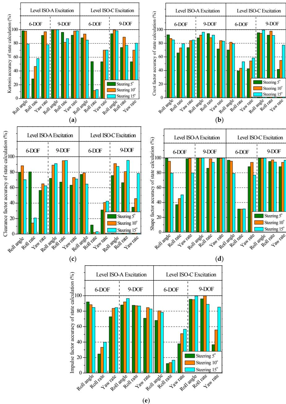
**Figure 12.** Accuracy of statistical features for vehicle state calculations using 6-DOF and 9-DOF models under road Level ISO-A/C excitation and steering wheel 5°, 10° and 15° conditions. (a) Kurtosis, (b) Crest factor, (c) Clearance factor, (d) Shape factor, (e) Impulse factor.
