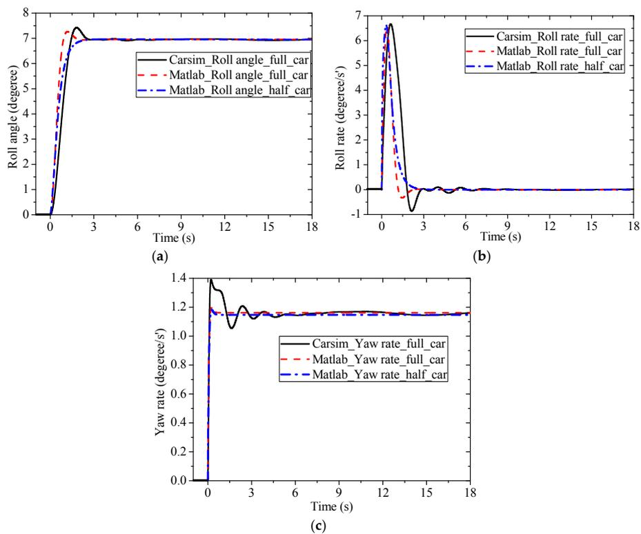
**Figure 9.** Results without road excitation (steering wheel angle was 10° at 80 km/h). (a) Roll angle; (b) Roll rate; (c) Yaw rate.
