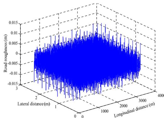
Figure 2. 3-D road roughness for Level ISO-A (at a velocity of 80 km/h).
