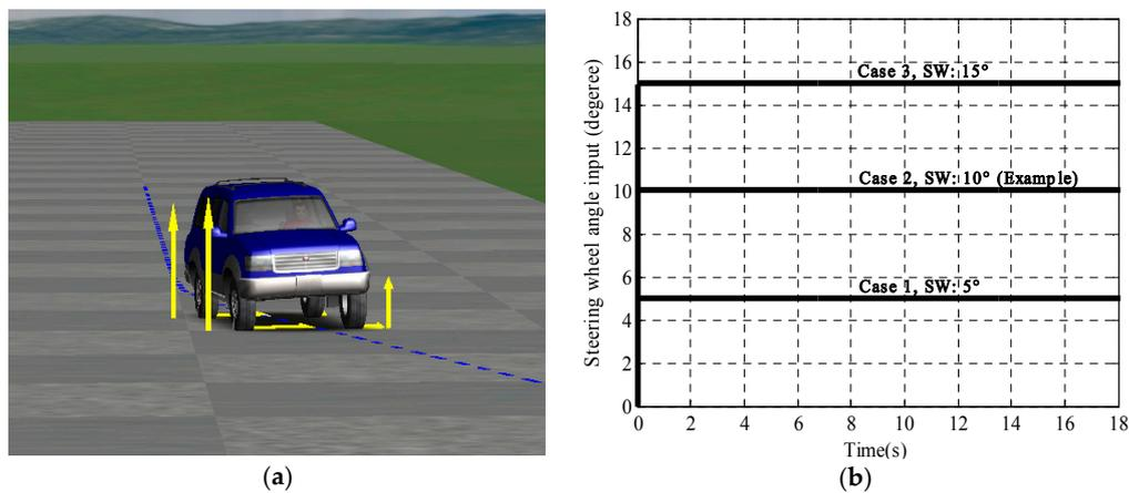
**Figure 8.** CARSIM simulation of roll behavior under various road excitation conditions. (a) Animation Screen. (b) Steering wheel input.
