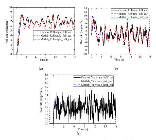
**Figure 11.** Results with road Level ISO-*C* excitation (steering wheel angle was 10° at 80 km/h). (a) Roll angle, (b) Roll rate, (c) Yaw rate.
