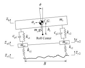
Figure 5. Half-car roll dynamics model.
