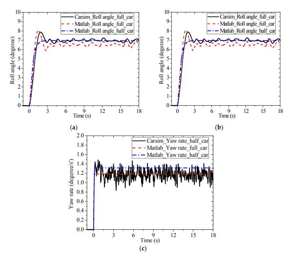
**Figure 10.** Results with road Level ISO-*A* excitation (steering wheel angle was 10° at 80 km/h). (a) Roll angle; (b) Roll rate; (c) Yaw rate.
