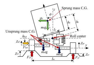
Figure 4. Roll behavior of vehicle system.
