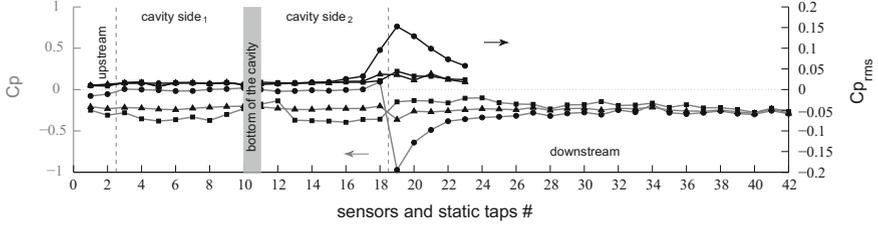
**Fig. 4** Mean- and rms-pressure spatial distribution for all the studied cases. Cavity side<sub>1</sub> denotes the leading side wall of the cavity and the cavity side<sub>2</sub> refers to the other side. Grey lines represent  $C_p$  (refers to the left axis) and black lines represent  $C_{p\ rms}$  (refers to the right axis)
