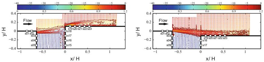
**Fig. 2** Vector plots of the mean-velocity magnitude ( $\|U\|/U_\infty$ —lower colorbar scale) and the mean-spanwise vorticity ( $\Omega_z^+ = \Omega_z \cdot H/U_\infty$ —upper colorbar scale). Cases I (left) and III (right). Vector lengths are normalized in order to enhance the visibility of the flow feature inside the cavity
