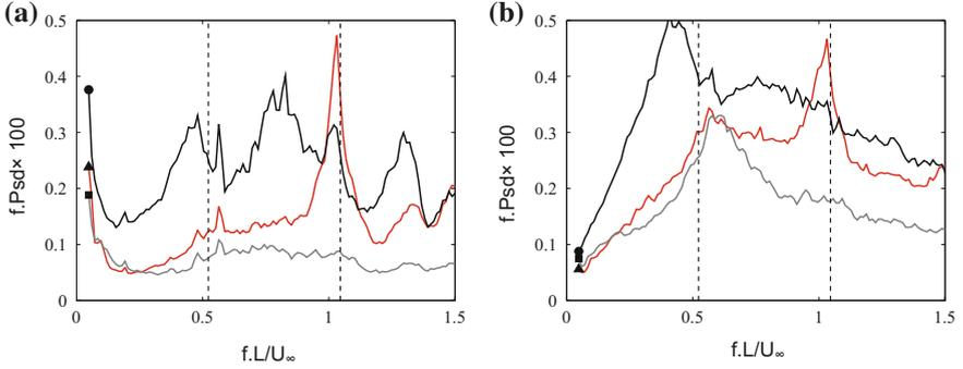
**Fig. 3** Premultiplied and normalized PSD of wall-pressure fluctuations (a) and (b) the *black dashed line* shows the first and the second modes from the Block's prediction with regard to the aspect ratio ( $\kappa = 0.57$ )
