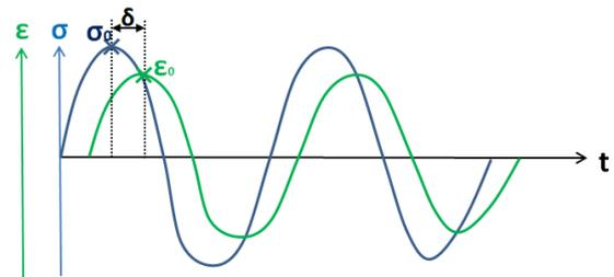
**Fig. 6.** Input and Output signal of a DMA test.
