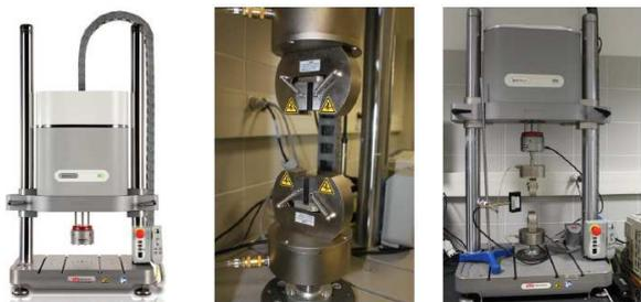
**Fig. 7.** Test device used for the DMA.
