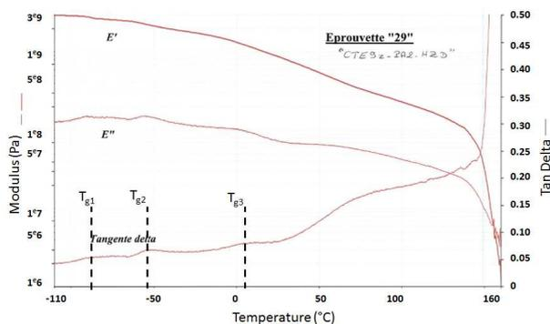
**Fig. 3.** Storage and loss modulus versus temperature – Heat from  $-110^\circ\text{C}$  to  $180^\circ\text{C}$  at  $3^\circ/\text{min}$ .
