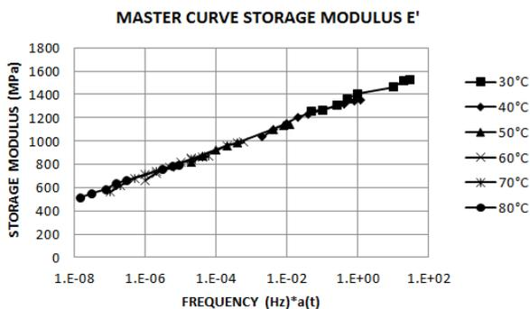
**Fig. 9.** Storage Modulus of the master curve versus frequency range \* shifted factors.
