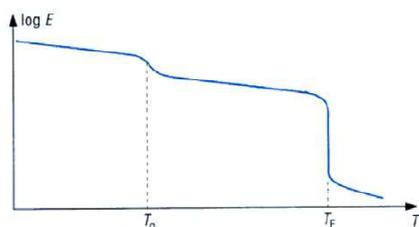
**Fig. 2.** Transition temperatures for a semi-crystalline [5].
