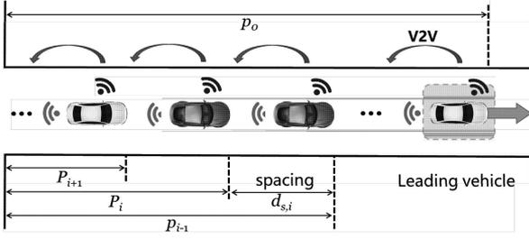
Fig. 1. A scenario and structure of vehicle platoons.
