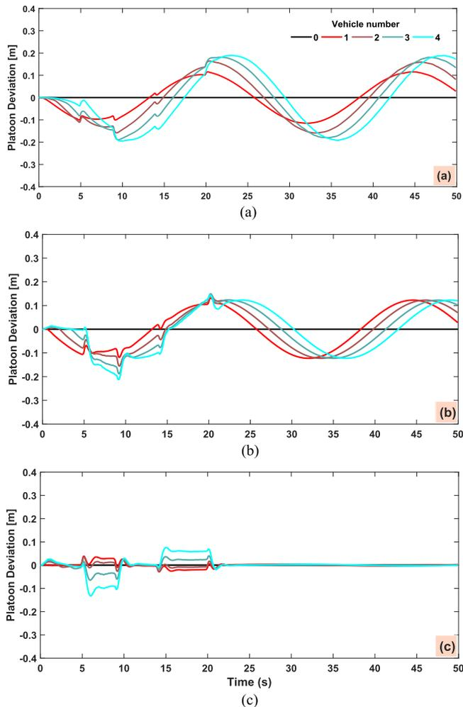
Fig. 15. Platoon deviation  $\Delta d_p$  (with PF communication topology). (a) Classical DMPC, (b) RN MPC in [30], (c) Proposed controller.
