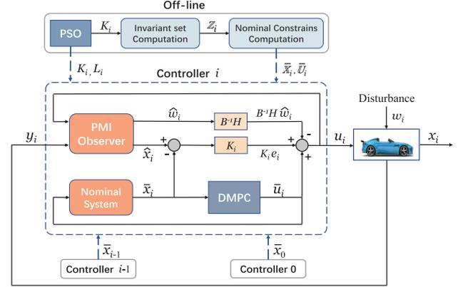
Fig. 3. Structure of the proposed integrated control scheme.
