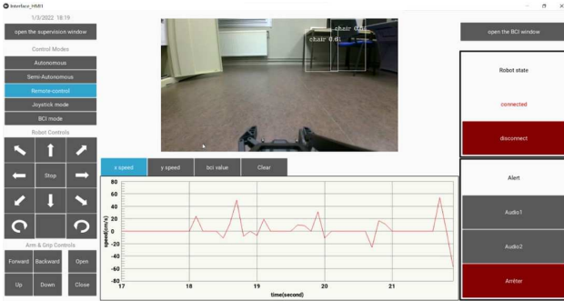
Fig. 6: Main HMI to support Human-BCI-Robot cooperation: selection of autonomous control (upper-left part), remote control (lower-left part), robot feedback (center part), connection (right part)
