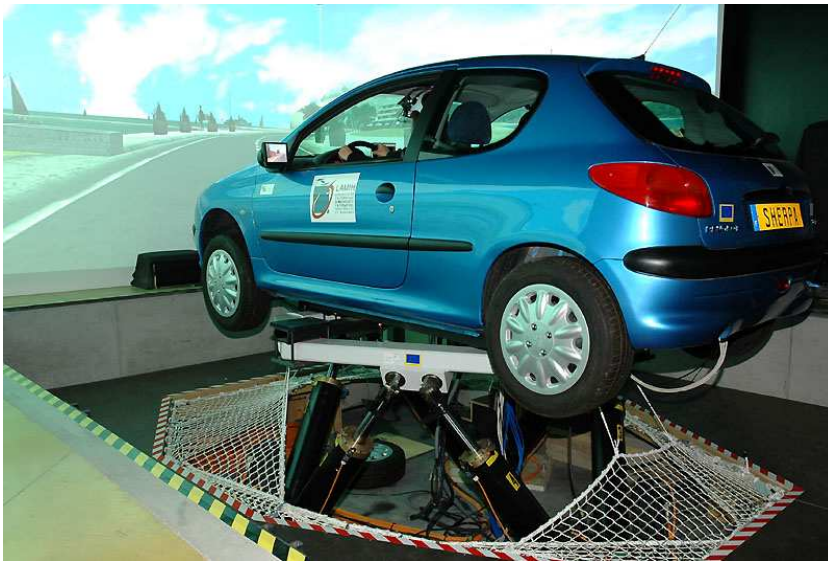
Figure 1. Driving simulator of the University of Valenciennes (SHERPA)
