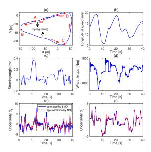
Fig. 9. Driving scenario 3: (a) vehicle trajectory X-Y, (b) longitudinal speed  $v_x$ , (c) steering angle  $\delta$ , (d) wheel torque  $T_w$ , (e) uncertainty  $d_1$  estimation and its NN-based approximation, (f) uncertainty  $d_2$  estimation and its NN-based approximation.
