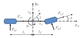
Fig. 1. Schematic of a two degrees-of-freedom vehicle model.
