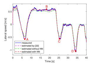
Fig. 8. Driving scenario 2: estimation of the lateral speed  $v_y$  by the TS fuzzy reduced-order observer with and without neural networks, as well as the observer [22].
