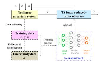
Fig. 2. Takagi-Sugeno fuzzy reduced-order observer structure with NN-based uncertainty identification (solid line: online computation, dashed line: offline computation).
