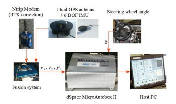
Fig. 4. Vehicle sensors and acquisition system.
