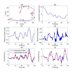
Fig. 5. Driving scenario 1: (a) vehicle trajectory X-Y, (b) longitudinal speed  $v_x$ , (c) steering angle  $\delta$ , (d) wheel torque  $T_w$ , (e) uncertainty  $d_1$  estimation and its NN-based approximation, (f) uncertainty  $d_2$  estimation and its NN-based approximation.
