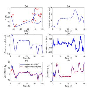
Fig. 7. Driving scenario 2: (a) vehicle trajectory X-Y, (b) longitudinal speed  $v_x$ , (c) steering angle  $\delta$ , (d) wheel torque  $T_w$ , (e) uncertainty  $d_1$  estimation and its NN-based approximation, (f) uncertainty  $d_2$  estimation and its NN-based approximation.
