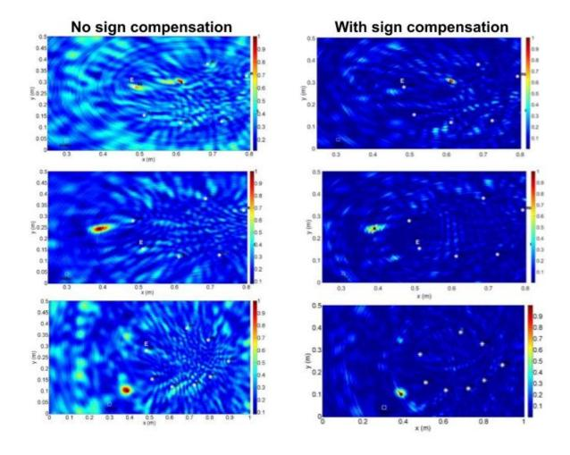
**Figure 4**. Imaging localization results at different defect locations at  $f_{pump}$ =1.5 Hz without random sign compensation (left column) and with it (right column).
