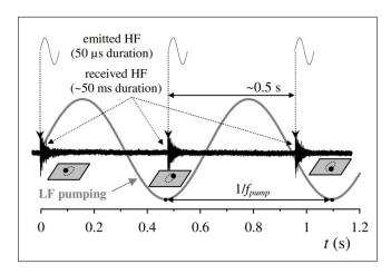
Figure 2. Typical pump-probe signals.
