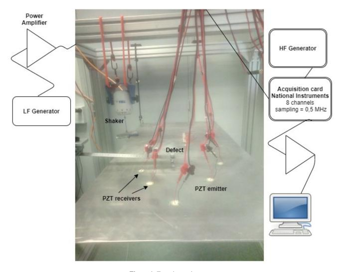
Figure 1. Experimental setup.
