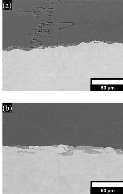
**Figure 1:** Morphology examples of Al/Cu interface MPW joint - obtained by scanning electron microscopy (SEM) (aluminum on top and copper on bottom in each picture) - (a) Planar and wavy interface morphology example for Al/Cu welded sample - (b) Vortex interface morphology example for Al/Cu welded sample
