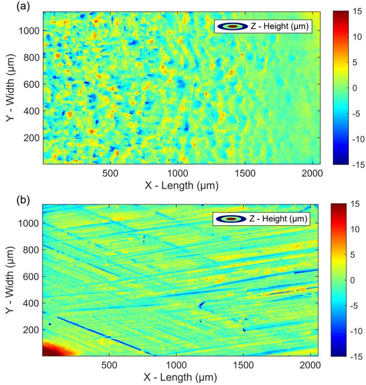
**Figure 8:** Topographic maps of interface after process analysis of XCT data - (a) Al/Cu interface topographic map located near welding zone end - (b) Air/Cu interface topographic map after grinding during sample preparation
