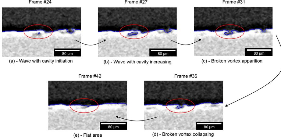
**Figure 12:** Broken vortex morphology evolution on width (Y-axis)
