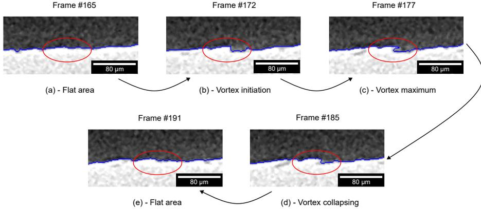
**Figure 11:** Standard vortex morphology evolution on width (Y-axis)
