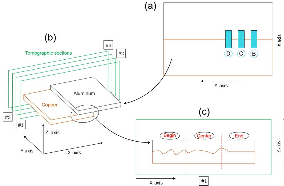
**Figure 6:** Sample position and coordinates base orientation of welding geometry and tomographic sections - (a) Cross-section sample position on global welding - (b) Tomographic section orientation for sample - (c) Position of different localizations (Begin, Center, End) for sample
