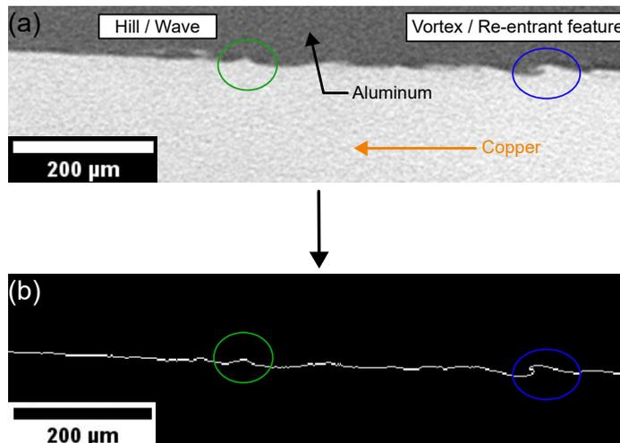
**Figure 5:** Example of transformed tomographic picture into binarized interface line with specific morphological elements - (a) Initial gray-level picture from X-Ray  $\mu$ -CT - (b) Binarized interface line
