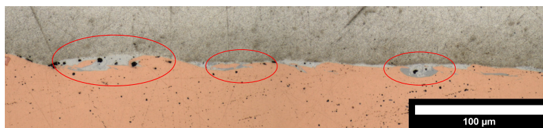
Figure 14: Stitched optical image from Al/Cu welded joint interface with highlighted broken vortex features at different stages
