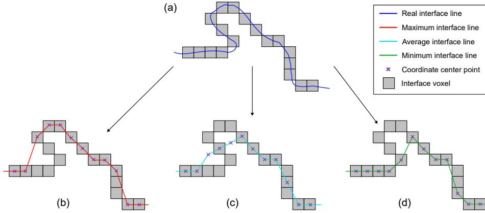
**Figure 9:** Scheme for variations in different height maps for vortex composed of interface voxels - (a) Real interface line with interface voxel - (b) Maximum interface line for maximum height map - (c) Mean interface line for average height map - (d) Minimum interface line for minimum height map
