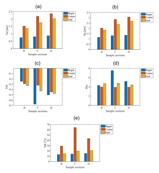
**Figure 10**: Plot of roughness parameters for different samples (B, C, and D) and localization (Begin, Center, End) for average height map - (a) Sa measurements - (b) Sq measurements - (c) Ssk measurements - (d) Sku measurements - (e) Sdr measurements
