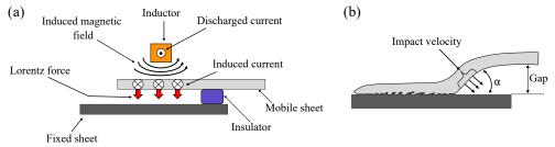
**Figure 3**: Scheme of the MPW process - (a) Definition of the parts and forces involved during the process - (b) Definition of the main process parameters
