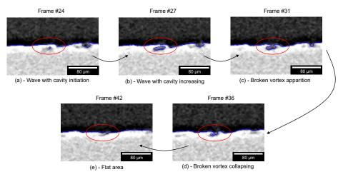
Figure 12: Broken vortex morphology evolution on width (Y-axis)
