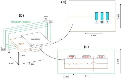
**Figure 6**: Sample position and coordinates base orientation of welding geometry and tomographic sections -(a) Cross-section sample position on global welding -(b) Tomographic section orientation for sample -(c) Position of different localizations (Begin, Center, End) for sample
