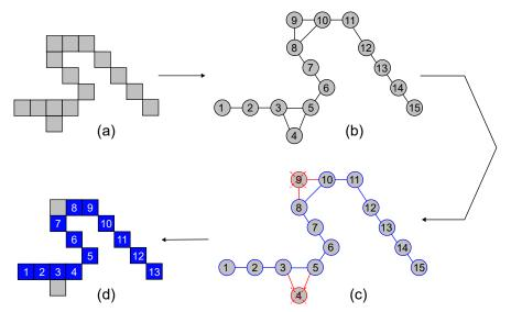
**Figure 7**: Scheme for presentation of graph network sequence - (a) Initial data input - (b) Graph network of previous pixel line - (c) Shortest path between first and last element - (d) Final extracted, ordered data
