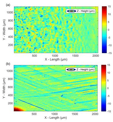
**Figure 8**: Topographic maps of interface after process analysis of XCT data - (a) Al/Cu interface topographic map located near welding zone end - (b) Air/Cu interface topographic map after grinding during sample preparation
