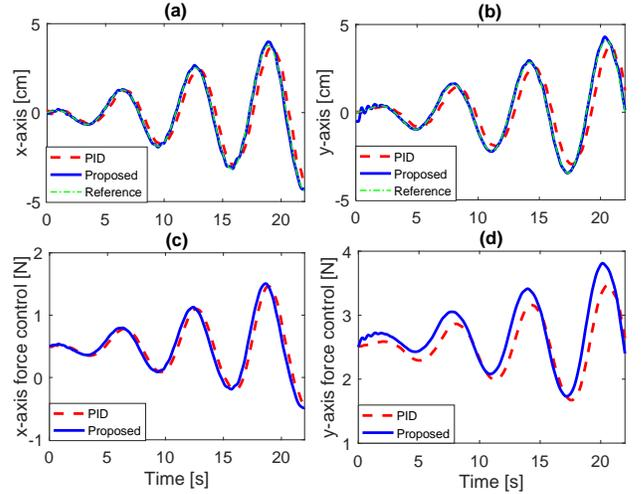
Fig. 13. Comparison of spiral trajectory tracking control. (a) Tracking performance along  $x$ -axis. (b) Tracking performance along  $y$ -axis. (c) Force control input in  $x$ -axis direction. (d) Force control input in  $y$ -axis direction.
