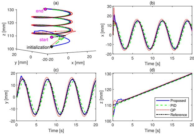
Fig. 8. Fast spiral trajectory tracking in Scenario 2.
