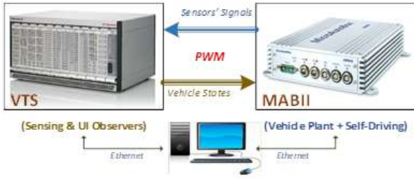
(a) Configuration of the HiL platform.
