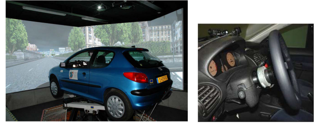
Fig. 2 SHERPA: dynamic LAMIH driving simulator (left), steering torque sensor (right)
