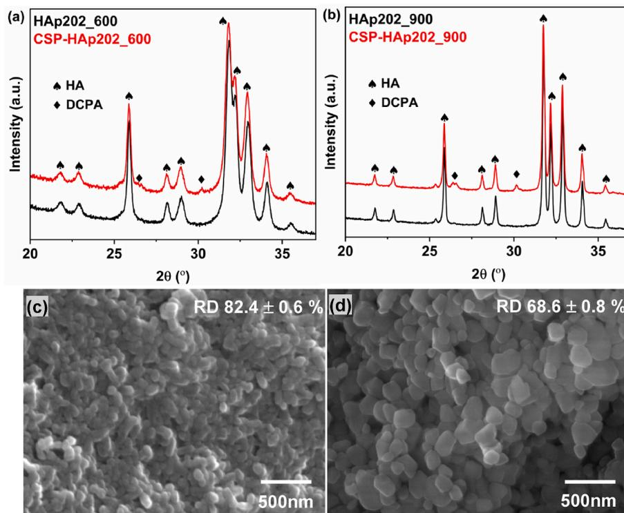
**Fig. 8.** (a & b) Comparative XRD patterns for the HAp202 calcined powders (600 & 900 °C) and cold sintered calcined HA powders at 200 °C using 2 M H<sub>3</sub>PO<sub>4</sub> solution respectively. Microstructure of cold sintered (c) HAp202\_600 powder, and (d) HAp202\_900 powder.
