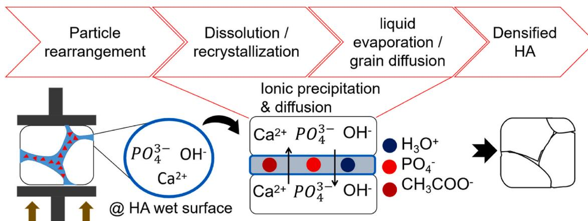
Fig. 4. Schematic illustration of the densification mechanism that occurs during the cold sintering of hydroxyapatite.
