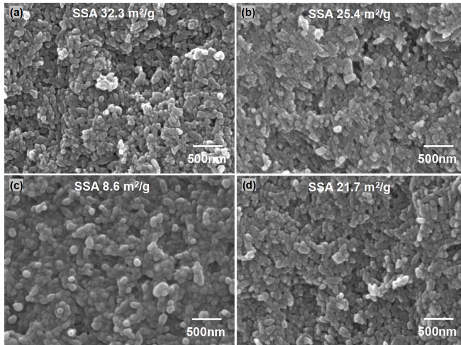
Fig. 6. SEM images of HAp202 powder cold sintered at 200 °C (a) without using liquids, (b) with H<sub>2</sub>O, (c) with 2 M H<sub>3</sub>PO<sub>4</sub> solution, and (d) with 2 M AcOH solution.
