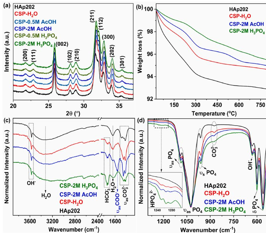
Fig. 7. (a) X-ray diffraction patterns of cold sintered HAp202 powder with H<sub>2</sub>O, (0.5 & 2 M) AcOH and H<sub>3</sub>PO<sub>4</sub> solution, (b) Thermogram of cold sintered HAp202 powder using H<sub>2</sub>O, 2 M AcOH & H<sub>3</sub>PO<sub>4</sub> solutions. FTIR patterns plotted (c) between wavenumber range 4000 to 1250 cm<sup>-1</sup>, and (d) between wavenumber range 1250 to 530 cm<sup>-1</sup>.
