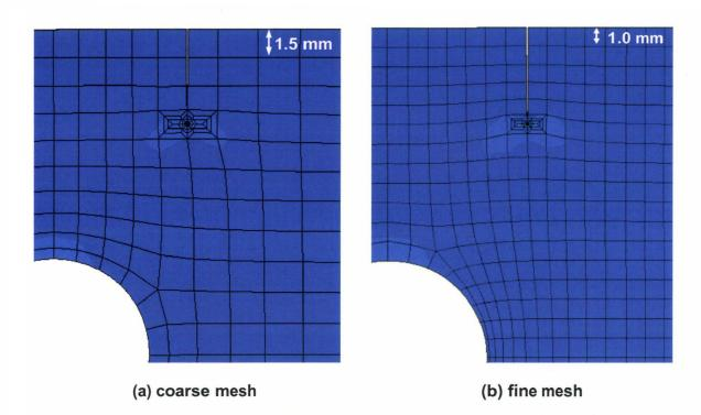
Fig. 84: Zencrack - Details of the coarse and fine FE models (initial crack length)
