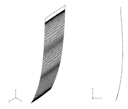
Fig. 87: Zencrack - Computed crack path (fine mesh)
