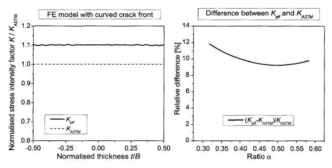
Fig. 74: (a) SIF along the crack front for a FE model with a curved front profile; (b) Relative difference between  $K_{eff}$  and  $K_{ASTM}$
