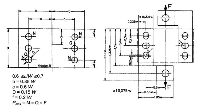
Fig. 66: Compact Tension Shear CTS specimen dimensions [Rich81]
