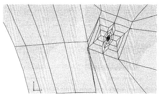
Fig. 86: Zencrack - Mesh distortion near the crack front (fine mesh)
