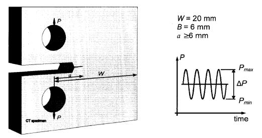
Fig. 64: Fatigue crack growth with CT specimen
