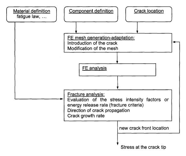
Fig. 45: Incremental crack propagation process
