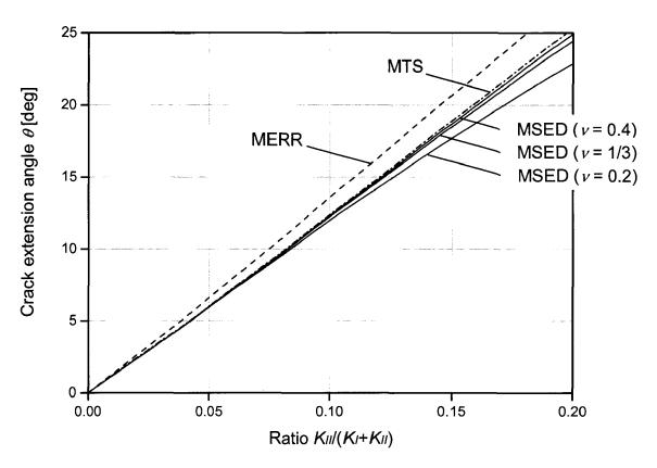
Fig. 30: MTS, MERR, MSED criteria for small ratios  $K_{II} / K_I$
