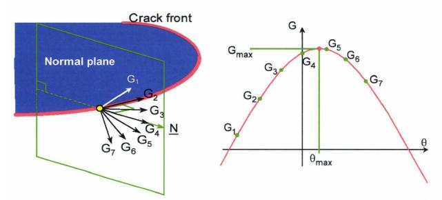
Fig. 48: Energy based calculation of G<sub>max</sub> and growth direction [Zen06]
