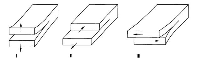
Fig. 4: Three modes of fracture: I, opening mode; II, sliding mode; III, tearing mode
