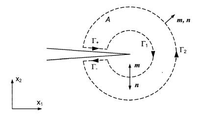
Fig. 18: Closed contour  $\Gamma_0$  around the crack tip
