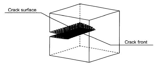
Fig. 1: Description of a crack tip
