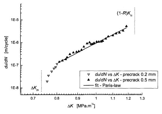
Fig. 119: Fatigue crack growth threshold (evaluation of  $\Delta K$  based on Eq. 142 [A-647])
