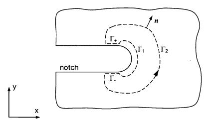
Fig. 16: Two-dimensional body containing a notch
