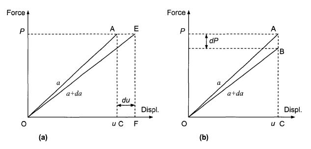
Fig. 8: Graphical representation of the energy release rate -Crack extension (a) under constant force; (b) under constant displacement
