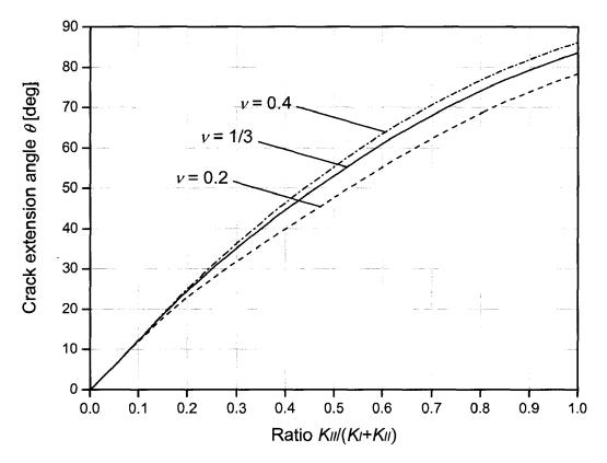
Fig. 28: MSED criterion - crack propagation angle  $\theta = f(K_{ll}/(K_l + K_{ll}))$
