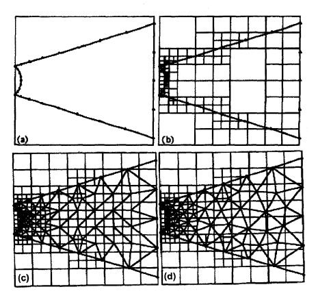
Fig. 49: Complete meshing using quadtree algorithms [Bit96]
