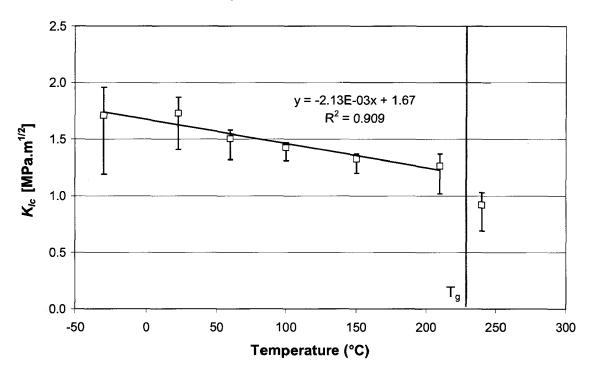
Fig. 100: Temperature dependence of  $K_{lc}$  for Mat4
