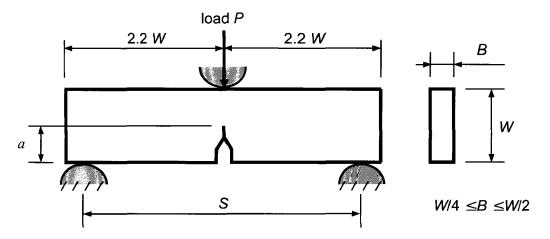
Fig. 61: Single Edge Notched SEN specimen dimensions
