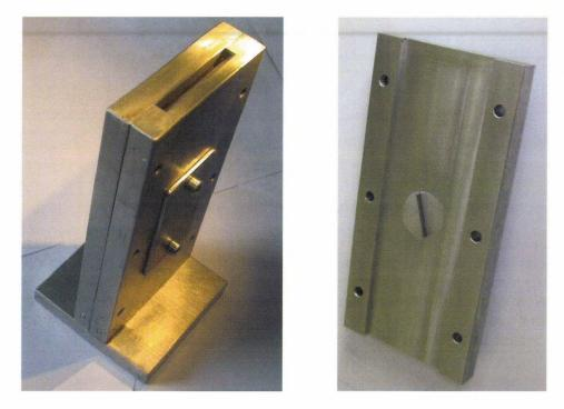
Fig. 102: a) Mould for CCT specimen; b) Inside part with adjustable blade orientation
