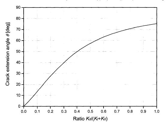
Fig. 27: MERR criterion - crack propagation angle  $\theta = f(K_{ll}/(K_l + K_{ll}))$
