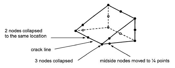
Fig. 38: 20-noded quarter point element [Aba05]
