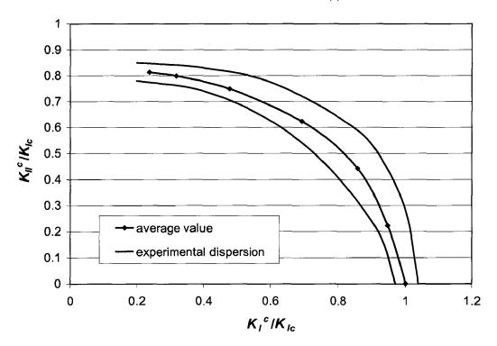
Fig. 109: Critical combinations ( $K_l^c$ ,  $K_{l'}^c$ ) according to experimental tests
