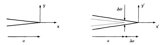
Fig. 14: Crack extension from *a* to  $a + \Delta a$
