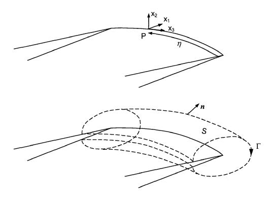
Fig. 19: J-integral in 3D: local coordinate system and closed surface
