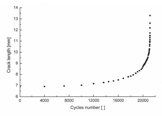
Fig. 113: Measured crack length
