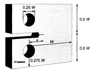
Fig. 59: Compact Tension specimen dimensions
