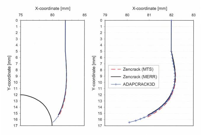
Fig. 89: Simulated crack path from ADAPCRACK3D and Zencrack: (a) real X-coordinates; (b) deformed X-coordinate
