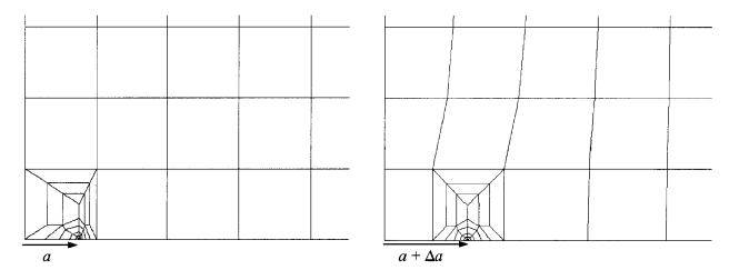
Fig. 58: Zencrack - Crack-block transfer [Zen06]
