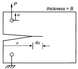
Fig. 7: Cracked plate subjected to an external load P
