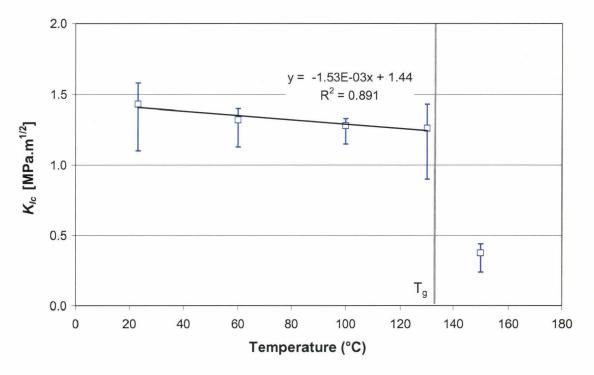
Fig. 99: Temperature dependence of  $K_{lc}$  for Mat2
