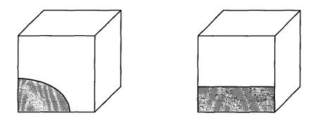
Fig. 55: Quarter circular or straight crack-block
