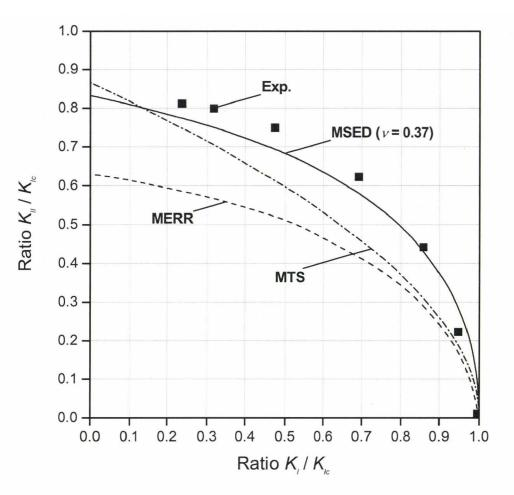
Fig. 110: Fracture criterion - Experiments and theoretical models
