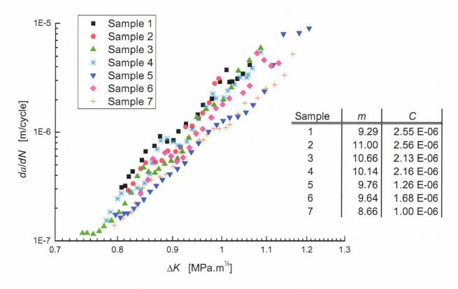
Fig. 117:  $da/dN - \Delta K$  curve and material coefficients for  $P_{max} = 110$  N with R = 0.1 (evaluation of  $\Delta K$  based on Eq. 142 [A-647])
