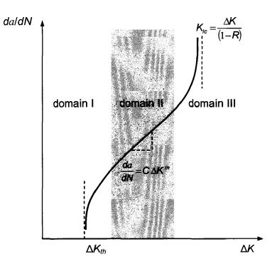
Fig. 65: Cyclic loading - Crack growth rate da/dN as a function of stress intensity factor range  $\Delta K$
