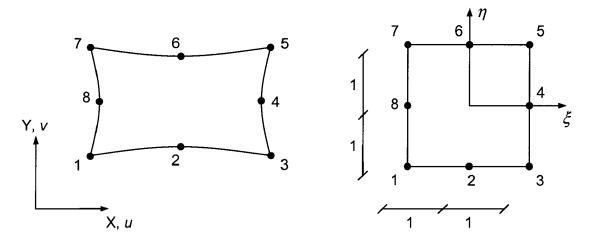
Fig. 34: 2D 8-noded isoparametric element
