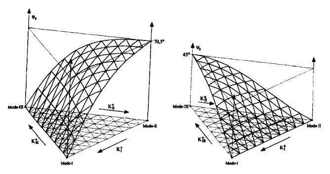
Fig. 24\*: Angle  $\theta_0$  and  $\psi_0$  depending on mixed-mode ratio [SFR01]
