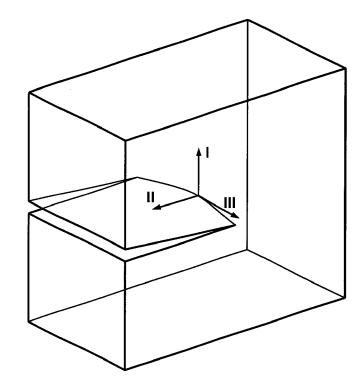
Mode I or opening mode: perpendicular to crack plane
