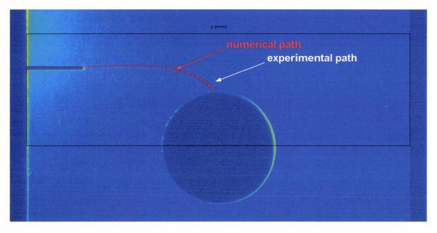
Fig. 112: Experimental and simulated crack path
