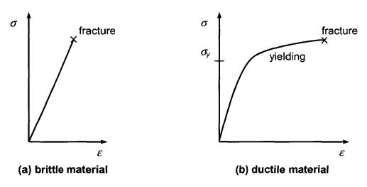
Fig. 2: Brittle and ductile material behaviour
