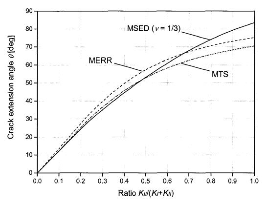
Fig. 29: Comparison between the MTS, MERR, and MSED criteria
