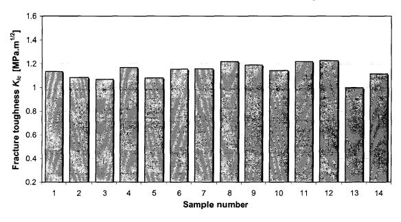
Fig. 90:  $K_{lc}$  measurement for Mat1 (ambient temperature) (evaluation of  $K_{lc}$  based on Eq. 138 [A-399])
