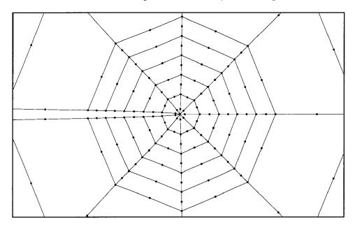
Fig. 37: Crack tip modelled with collapsed 8-noded quarter point elements
