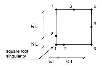
Fig. 35: 8-noded quarter point element
