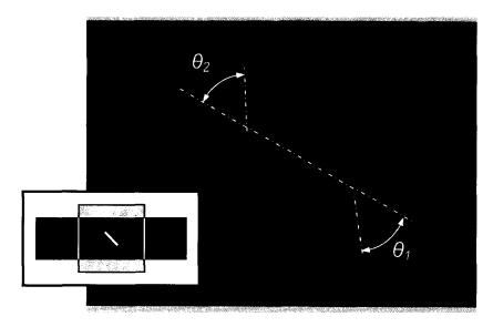
The direction of crack propagation is optically measured at the fractured specimen.
