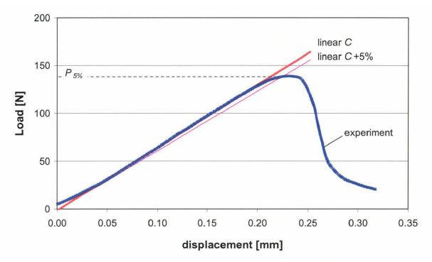
Fig. 98: Load-displacement curve for Mat2 at T = 130°C
