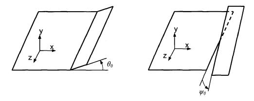
Fig. 22: Crack propagation angles  $\theta_0$  and  $\psi_0$
