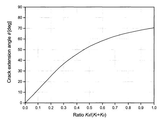
Fig. 25: MTS criterion - crack propagation angle  $\theta = f(K_{ll}/(K_l + K_{ll}))$
