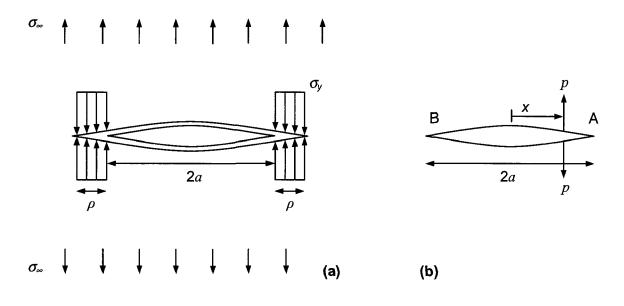
Fig. 21: a) Dugdale's plastic zone model b) Wedge forces
