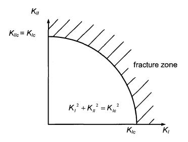
Fig. 31: Mixed-mode loading - Schematic representation of fracture zone
