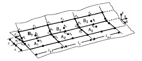
Fig. 44: VCCT - 27-noded brick element model [JiM03]
