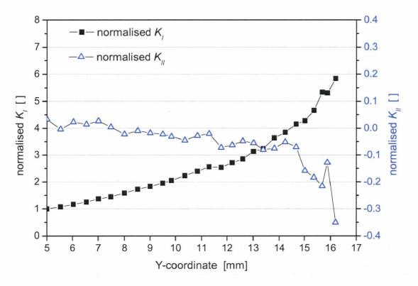
Fig. 83: ADAPCRACK3D - Normalised  $K_l$  and  $K_{ll}$  as function of the Y-coordinate (normalised by  $K_l$  at the first increment)
