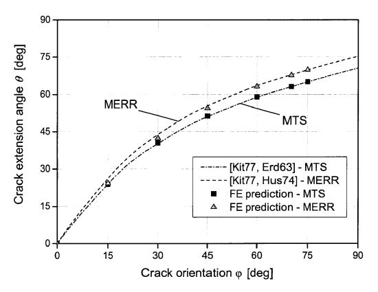
Fig. 77: CCT specimen - Prediction of the crack propagation direction
