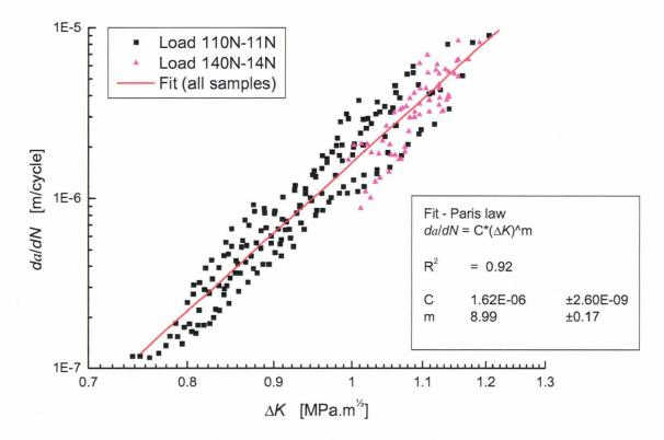
Fig. 118: Fitting of experimental data with R = 0.1 under  $P_{max} = 110$  N and  $P_{max} = 140$  N (evaluation of  $\Delta K$  based on Eq. 142 [A-647])
