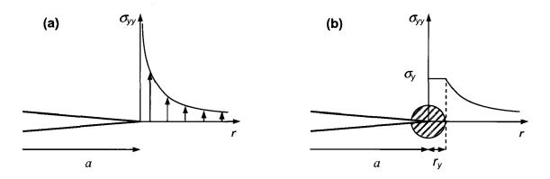
Fig. 3: a) Shear stress distribution at the crack tip for ideal elastic material behaviour; b) Irwin's plastic zone [Gro96]
