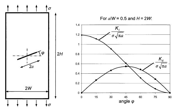
Fig. 67: Centre cracked tension CCT specimen [Wil71, Kit77, Mur87]
