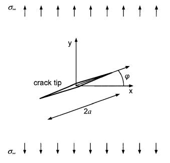
Fig. 129: Infinite plate with a slant crack under a uniform uniaxial tensile stress
