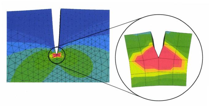
Fig. 53: Submodeling technique- Global model and associated submodel
