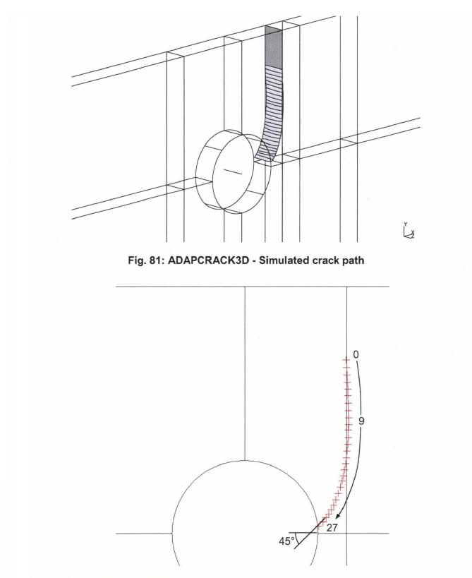
Fig. 82: ADAPCRACK3D - Projection of the crack front on the X-Y plane (from initial state 0 to increment 27)
