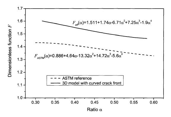
Fig. 75: Dimensionless functions  $F_{ASTM}$  and  $F_{eff}$  (from FE models of CT specimen with B = 6 mm and W = 20 mm, v = 0.37)
