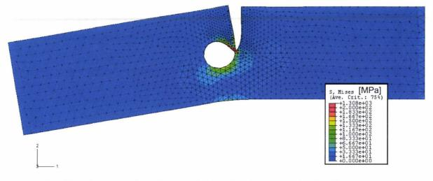
Fig. 80: Global model - Stress distribution in perforated SEN specimen after 27 increments (von Mises stress [MPa], deformation factor = 50)
