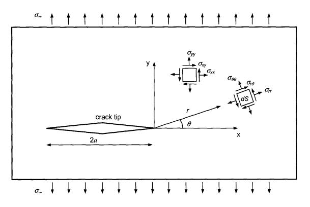
Fig. 9: Coordinate system and stresses in the near-tip region of a crack
