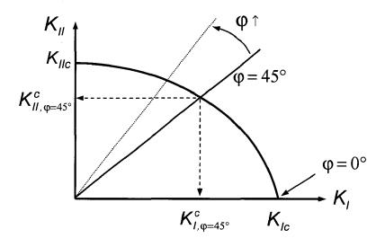
Fig. 108: Mixed-mode loading - Design of fracture criterion
