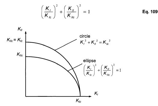
Fig. 32: Mixed-mode loading - Empirical fracture criteria
