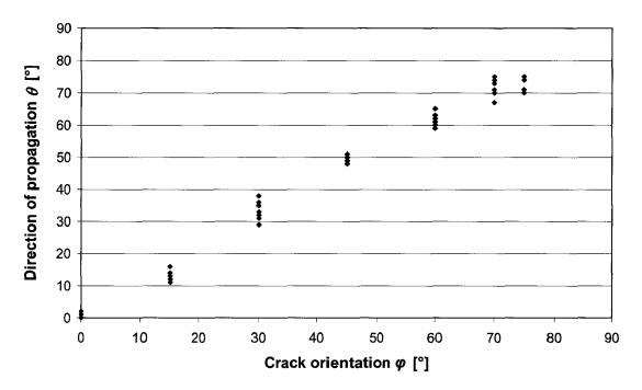
Fig. 105: Angle of crack propagation measured on CCT specimens  $\theta = f(\varphi)$
