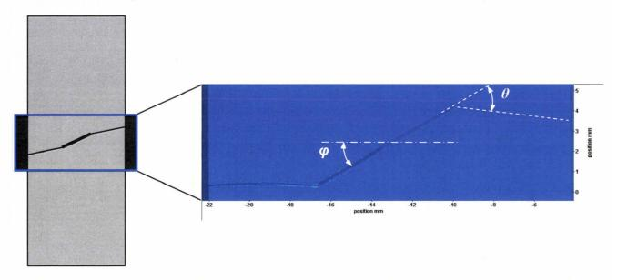
Fig. 103: Crack orientation  $\varphi$  and direction of crack propagation  $\theta$
