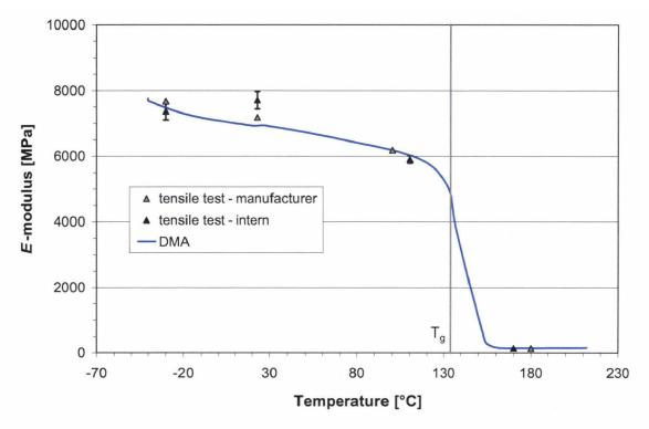
Fig. 97: Temperature dependence of the *E*-modulus for Mat2
