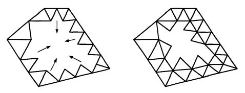
Fig. 50: Complete meshing using advancing front algorithm
