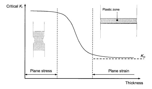
Fig. 13: Effect of specimen thickness on  $K_{lc}$
