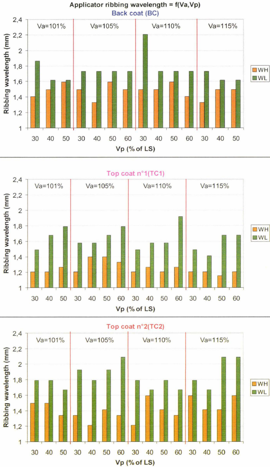
Figure 2-16: Ribbing wavelength as a function of rolls speeds, Two load cases, three paints: BC, TC1 and TC2
