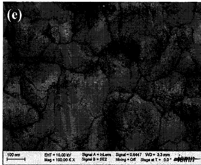
Fig. 6.1. Scanning electron microscope (SEM) photographs of the surface of (Ba,Sr)TiO 3 (BST) thin films: (a) 45 nm, (b) 100 nm, (c) 200 nm, (d)415 nm, and (e) 800 nm, respectively.
