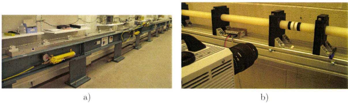
Figure 2.7: a) pre-stressed tensile and b) visco-elastic compressive Hopkinson bars.
