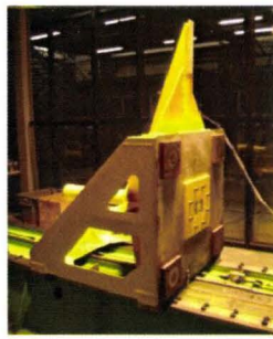
Impactor (mass 350 Kg) speed 16 m/s
