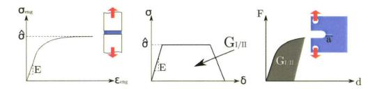
Figure 4.7: cohesive elements properties identification.
