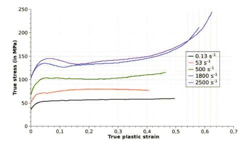
Figure 2.35: true stress versus true plastic strain for 4 MPa curing pressure specimen.
