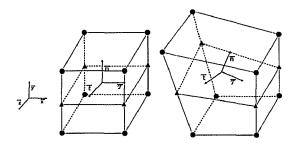
Figure 4.11: illustration of local basis.
