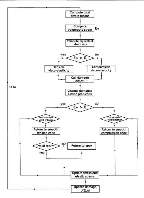
Figure 3.19: algorithm of the implemented behaviour model.
