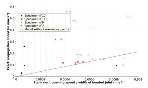
Figure 4.43: crack propagation speed in function of the normative variable.
