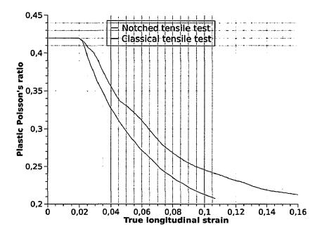
Figure 2.42: evolution of plastic Poisson's ratio.
