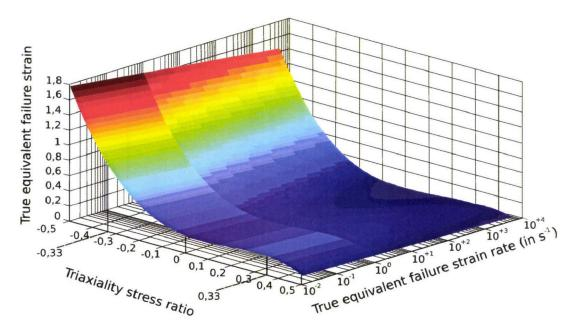
Figure 2.60: 3D representation of the new failure criterion.
