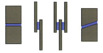
Figure 2.1: Classical bonded joints geometries.
