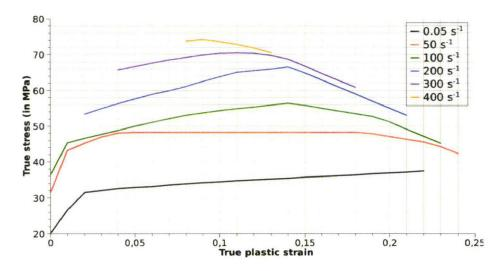
Figure 2.34: true stress / true plastic strain curves obtained with  $SE\bar{E}$  method.
