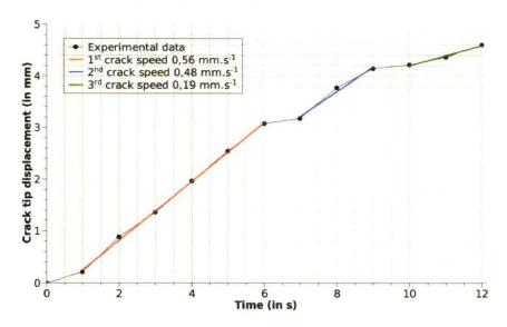
Figure 4.42: crack propagation speed identification.
