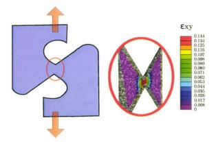
Figure 6.1: illustration of new shear specimens for polymeric materials.
