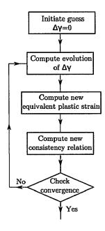
Figure 3.16: Newton Raphson algorithm schema.
