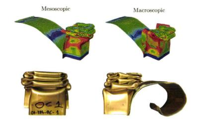
Figure 5.28: deformed shapes for both numerical models and experiments.
