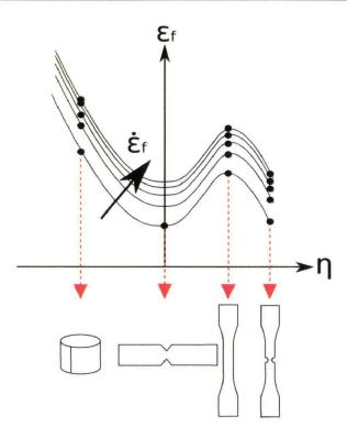
Figure 2.57: identification strategy for the failure criterion.
