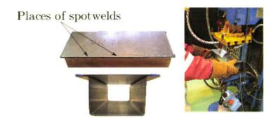
Figure 5.24: spotweld machine and places for spotweld.
