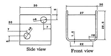
Figure 4.28: geometry of the double U specimens.
