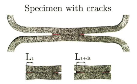
Figure 4.38: crack tip displacement identification.
