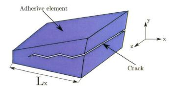
Figure 4.17: illustration of crack propagation through an element.
