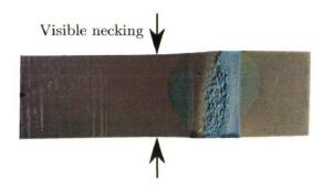
Figure 3.1: example of necking in a steel single lap joint test.
