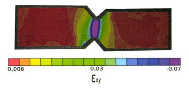
Figure 2.25: shear strain contour plot for a Iosipescu shear specimen.
