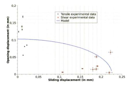
Figure 4.37: identification of the failure initiation criterion.
