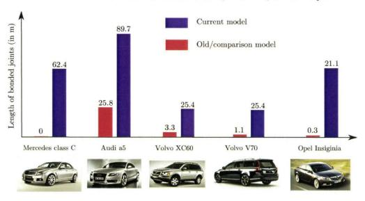
Figure 1.1: evolution of structural bonding use in some car models
