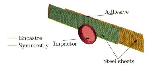
Figure 5.14: dynamic flexure simulation setup.
