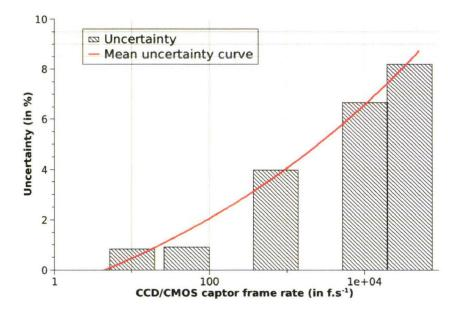
Figure 2.23: computed uncertainty for the various frame acquisition rate.
