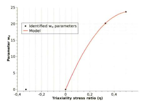
Figure 2.56: identification of  $w_d$  damage evolution law parameter.
