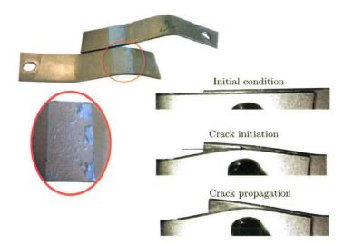
Figure 5.20: experimental crack initiation on the dynamic flexure test.
