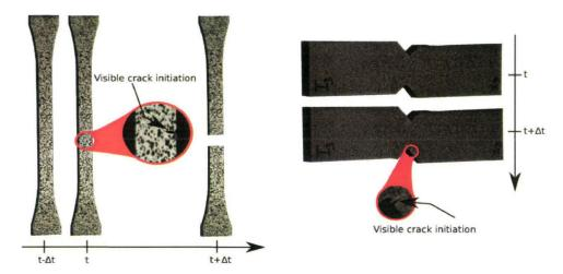
Figure 2.22: failure detection technique used for tensile, notched tensile and shear tests.
