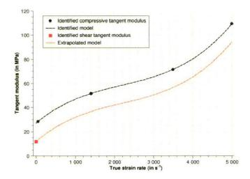
Figure 4.27: identification of tangent moduli in macroscopic approach.
