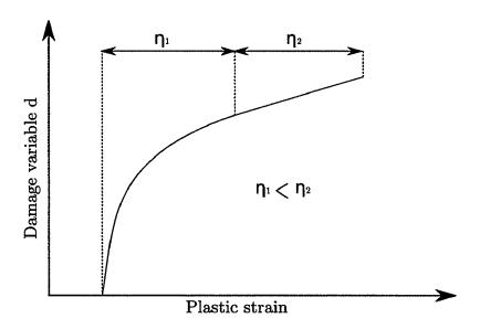
Figure 3.18: illustration of damage update technique.
