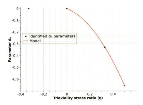
Figure 2.54: identification of  $d_0$  damage evolution law parameter.
