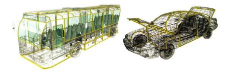
Figure 1.4: possible places of structural bonding in transportation structures (yellow lines).
