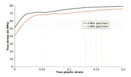
Figure 2.37: influence of curing pressure on the stress level of toughened epoxy  $(53 \text{ s}^{-1})$ .
