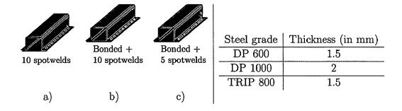
Figure 1.2: crashbox configurations a) 10 spotwelds, b) 10 spotweld + bonding and c) 5 spotwelds + bonding and thicknesses for the corresponding steel grade.
