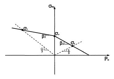
Figure 3.9: illustration of the double Drucker Prager yield criterion.
