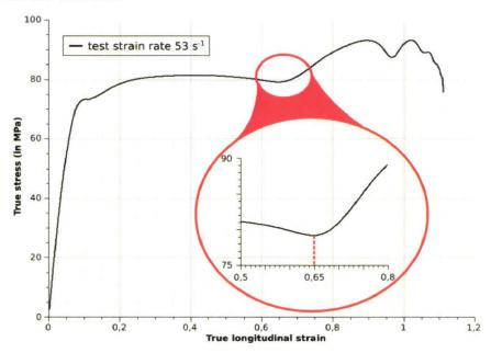
Figure 2.21: failure detection technique for compressive tests.
