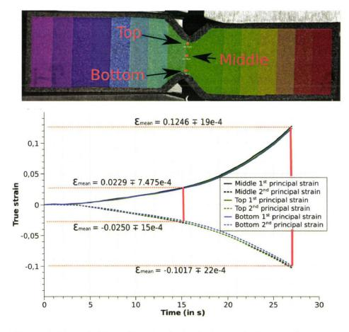
Figure 2.40: evolution of local principal strains during an shear test.
