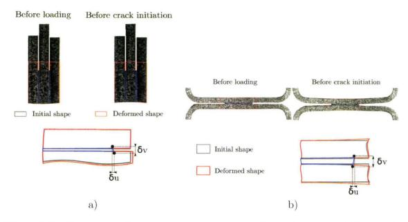
Figure 4.32: illustration of measurement protocol for a) tensile tests and b) shear tests.
