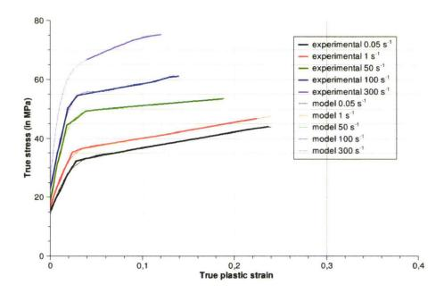
Figure 2.50: identification of tensile behaviour law.
