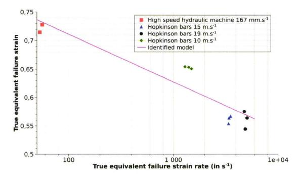
Figure 2.48: evolution of equivalent failure strain of compressive specimens in function of the equivalent strain rate.
