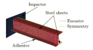
Figure 5.25: dynamic axial crushing simulation setup.
