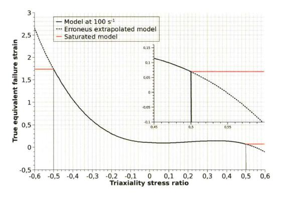
Figure 2.63: failure criterion saturation in term of triaxiality stress ratio.
