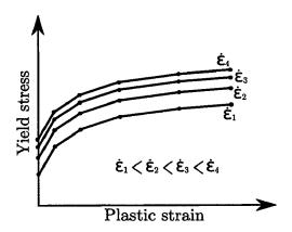
Figure 3.6: illustration of tabulated visco-plastic behaviour law.
