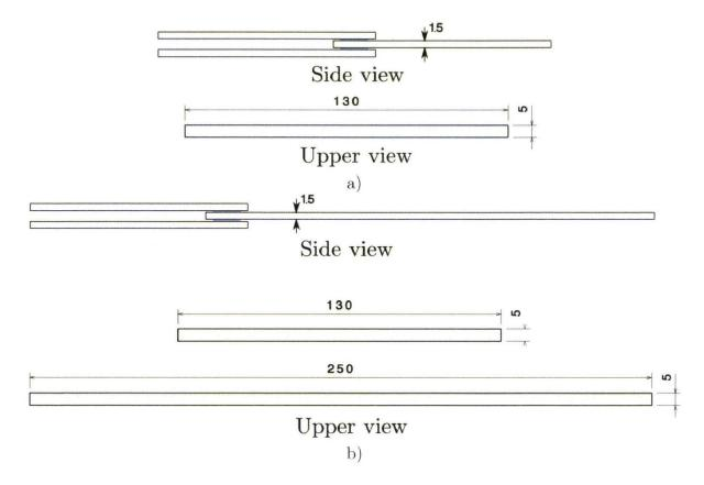
Figure 4.29: geometry of the double lap joints specimens a) in static and b) in dynamic.
