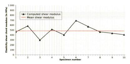
Figure 2.30: computed elasticity shear chord modulus.
