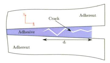
Figure 4.39: illustration of the crack tip displacement measurement.
