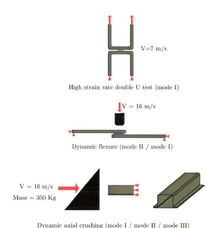
Figure 5.1: description of experiments and load complexity.
