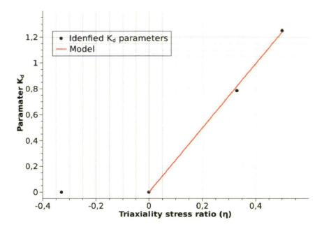
Figure 2.55: identification of  $K_d$  damage evolution law parameter.
