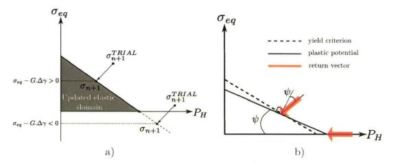
Figure 3.13: a) selection of the appropriate return vector and b) resulting return vectors.
