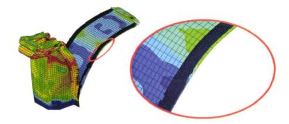
Figure 5.31: numerical failure facies of only bonded crashboxes.
