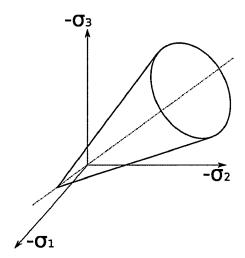
Figure 3.11: 3D representation of the plastic potential.
