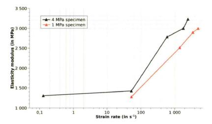
Figure 2.29: evolution of compressive elasticity modulus in function of strain rate and curing pressure.
