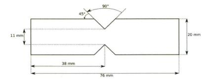
Figure 2.15: normalized geometry of the Iosipescu shear specimen.
