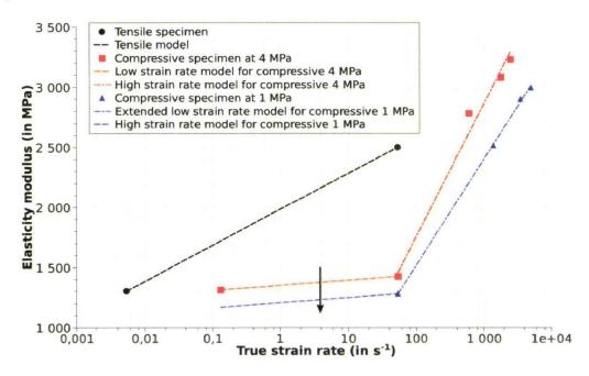
Figure 2.49: evolution of elasticity modulus in function of true strain rate.
