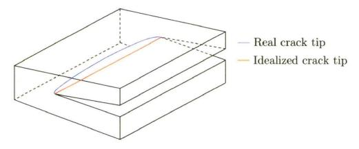
Figure 4.40: idealization of the crack tip.
