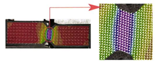
Figure 2.39: principal directions of diagonalized strain tensor.
