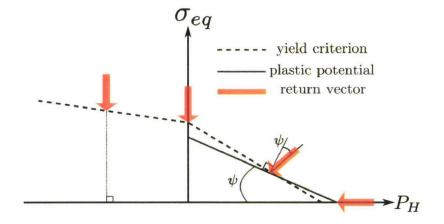
Figure 3.14: return vectors for the tensile, shear and compressive cases.
