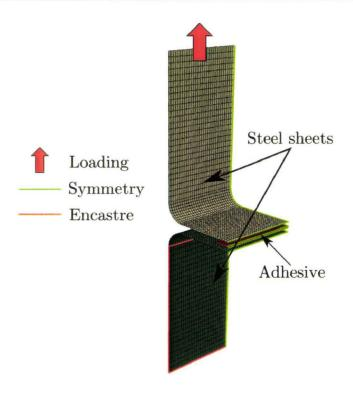
Figure 5.7: FE model of the double U test.
