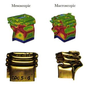
Figure 5.34: deformed shapes for both numerical models and experiments.
