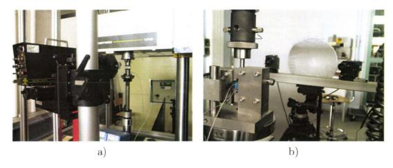
Figure 2.17: configuration of a) electro-optical extensometer and b) 3D DIC.
