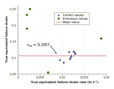
Figure 2.47: true equivalent failure strain on Iosipescu shear tests.
