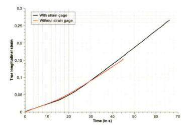
Figure 2.28: influence of strain gage on the true longitudinal strain in center of specimens.
