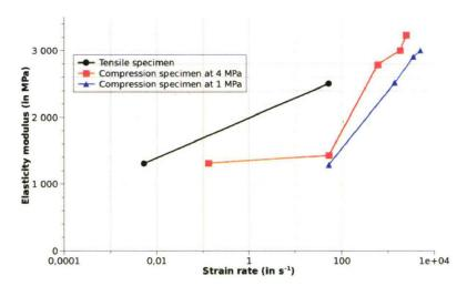
Figure 2.32: synthesis on the elastic moduli measurements.
