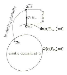
Figure 3.15: illustration of closed point method.
