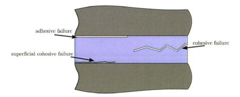
Figure 3.3: different failure modes in a bonded joint.
