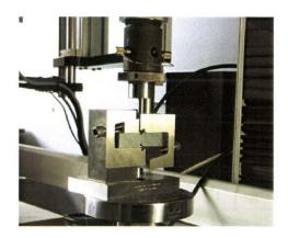
Figure 2.8: Iosipescu shear test device.
