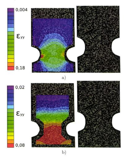
Figure 2.24: a) true longitudinal strain field with a  $8\mu$ m strain length calculation and b) true longitudinal strain field with a  $300\mu$ m strain length calculation.
