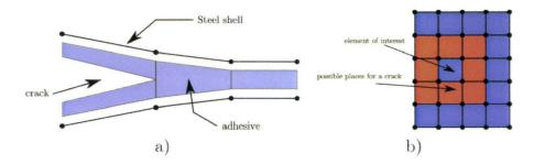
Figure 4.22: schematic representation of boundaries tests a) in face and b) in normal plane of the bonded joint.
