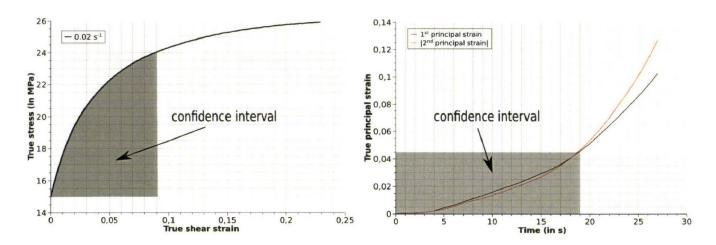
Figure 2.41: shear behaviour law and confidence interval.
