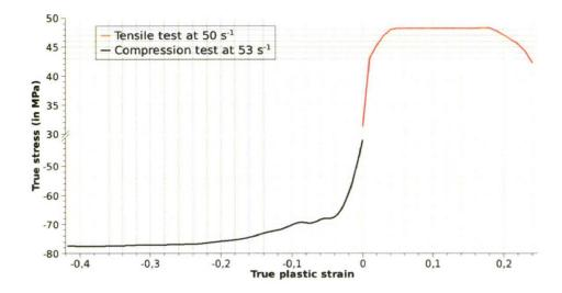
Figure 2.44: comparison between tensile and compressive plasticity behaviour.
