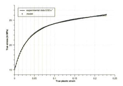
Figure 2.51: identification of shear behaviour law.
