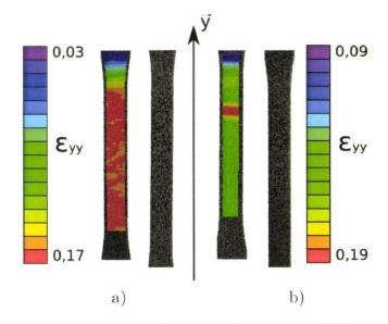
Figure 2.3: difference on strain fields between a) a pore and b) a pore-free specimen.
