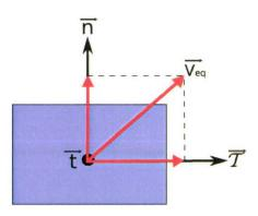
Figure 4.18: equivalent loading speed.
