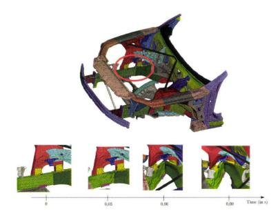
Figure 5.41: detailled view of the cup shock - crashbox link.
