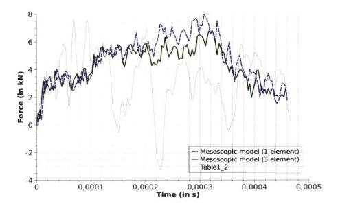
Figure 5.18: effect of the mesh refinement through thickness.
