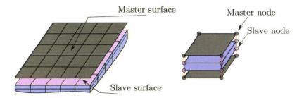
Figure 5.2: numerical link between steel and adhesive.
