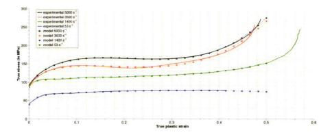
Figure 2.52: identification of compressive behaviour law.
