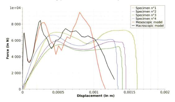
Figure 5.9: experimental and numerical force displacement curves.
