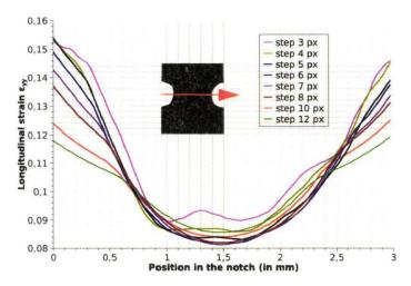
Figure 5.4: effect of step size on the failure strain computation in D.I.C.
