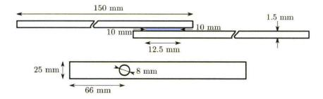
Figure 5.13: geometries of the specimen.
