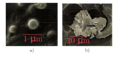
Figure 1.6: a) polymer nodules and b) mineral compounds.
