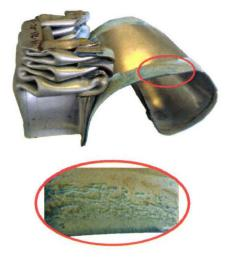
Figure 5.30: experimental failure facies of only bonded crashboxes.
