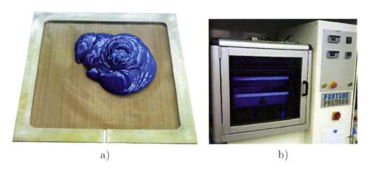
Figure 2.2: description of a) aluminum mould and b) heating press.
