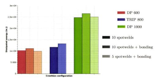
Figure 1.3: evolution of dissipated energy in function of the crashbox configuration.
