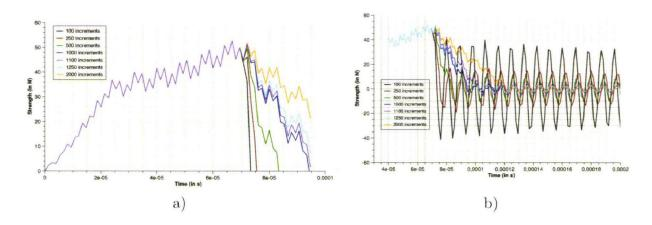
Figure 4.20: reaction force a) until crack propagation through the element and b) after the failure of the element.
