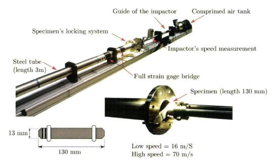
Figure 5.12: presentation of the ballistic device.
