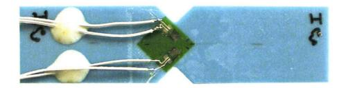
Figure 2.16: strain gages on Iosipescu specimen.
