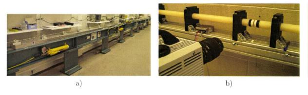
Figure 2.7: a) pre-stressed tensile and b) visco-elastic compressive Hopkinson bars.
