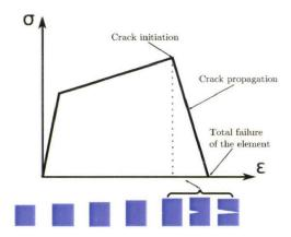
Figure 4.9: crack propagation through an element.
