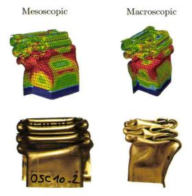
Figure 5.36: deformed shapes for both numerical models and experiments.
