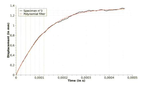
Figure 5.16: filtering of the displacement of the impactor.
