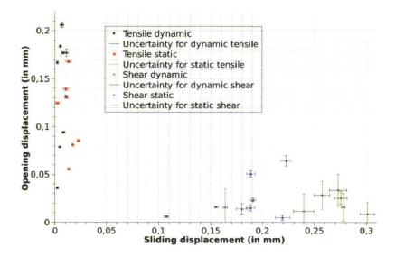
Figure 4.34: results in terms of opening and sliding displacements for the different strain rates.
