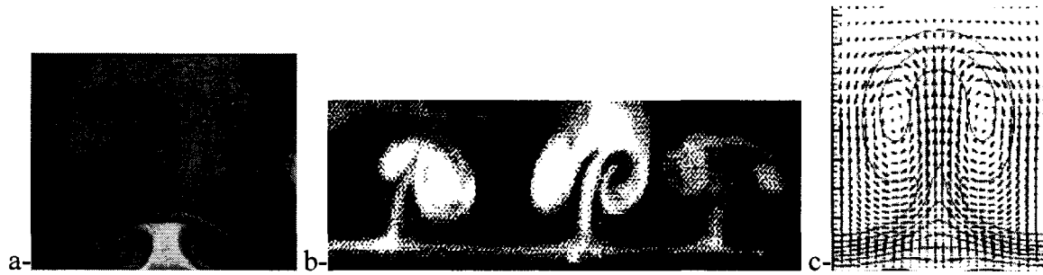
Figure 13 : Görtler instabilities experimentally observed a-[Camci, 2002], b-[Ligrani, 2000] and numerically calculated c-[Girgis, 2002].
