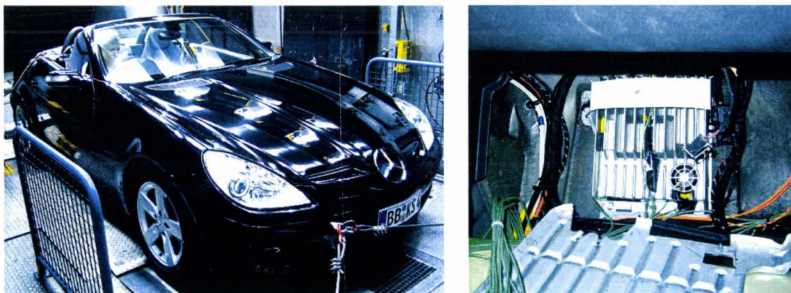
Figure 5.18. Sound amplifier in a compartment under the passenger's feet; experimental set-up.
