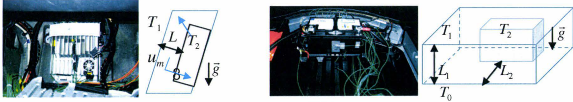
Figure 3.2. Characteristic dimensions for convection around a sound amplifier (left) and a lead-acid battery (right) assembled in a vehicle.
