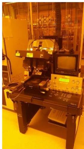
Figure 2.17 : Aligner MA6/BA6 Suss Micro Tec.
