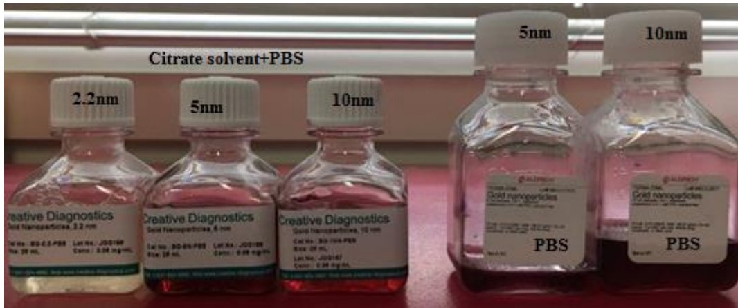
Figure III.1. Gold nanofluids of different sizes (2, 5 and 10 nm) and coating solutions (PBS and Citrate).
