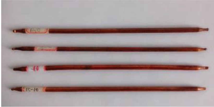
Figure I.15. Photograph of the four miniature heat pipes.
