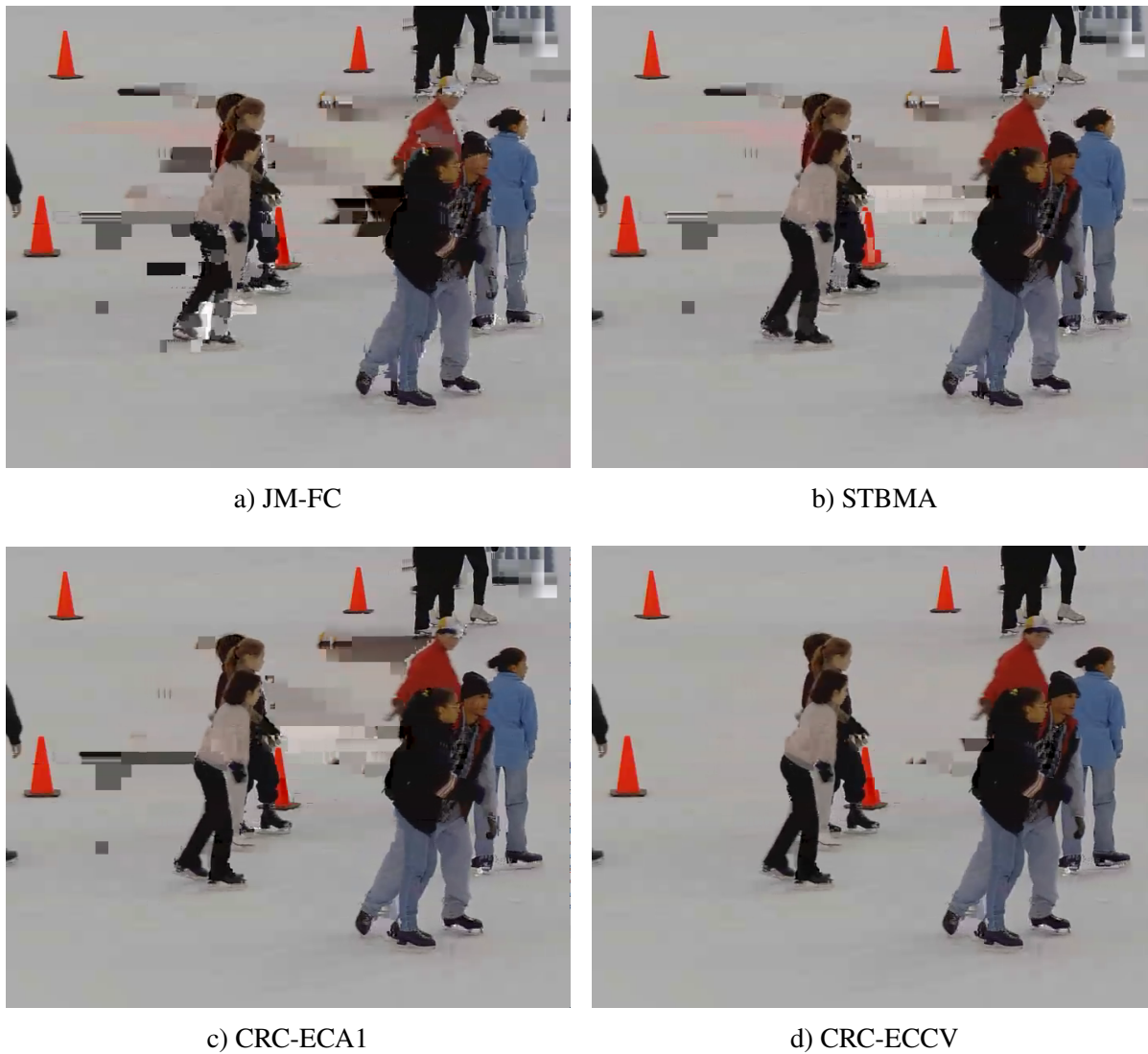
Figure 4.10 Visual comparison of the literature methods to the proposed approach on AVC encoded Ice sequence (4CIF) at QP32 for an E_b/N_0 value of 8 dB.
