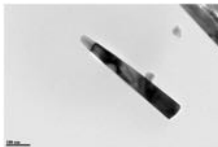
Figure 8. TEM image of ZnO nanorods scraped from fabric.
