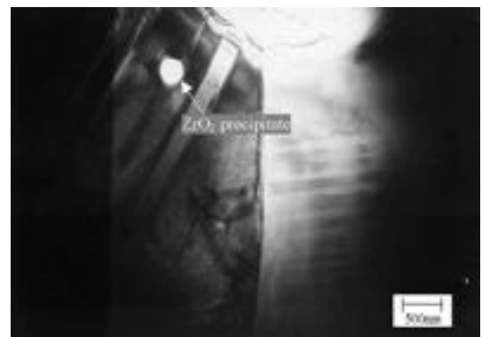
Fig. 3. STEM observation of ceramic C–Ni. Specific precipitation of zirconia is identified.
