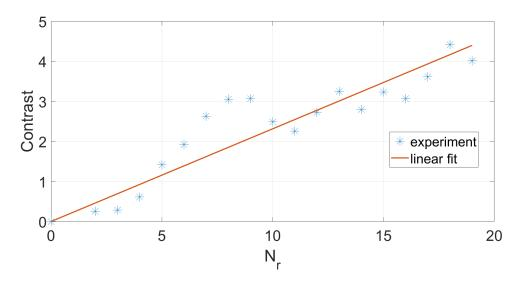
FIGURE 4.12 – Dependency of image contrast on number of receivers.
