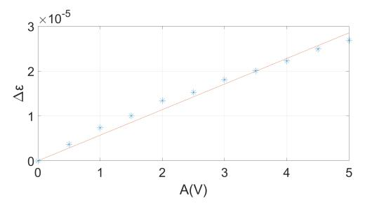
FIGURE 2.6 – Acoustical strain in the center of sphere-plate contact as a function of pump amplitude.
