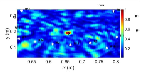
FIGURE 4.10 – Passive dynamic reference-free localization image of a CAN obtained with  $N_s = 18$  noise emitters and  $N_r = 19$  receivers. Defect is located at (0.66,0.185) m.
