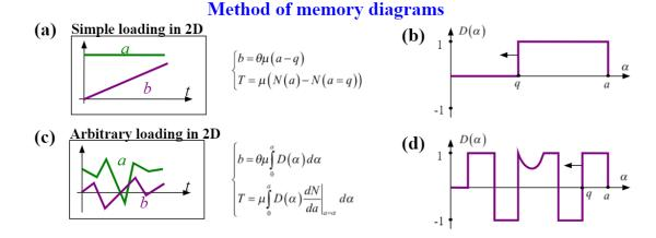
FIGURE 5.4 – Examples of memory diagrams (b) and (d) for simple (a) and complex (c) loading protocols, respectively. For the simple case, load-displacement relationship is known, for the complex one, method of memory diagrams is applied to find it.
