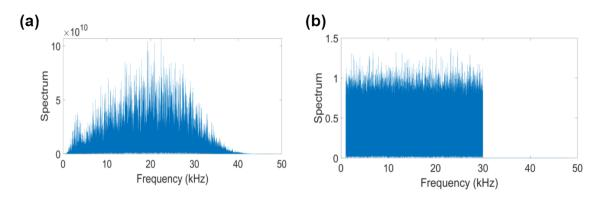
FIGURE 4.3 – Spectrum of the received signals : (a) before and (b) after the whitening procedure.
