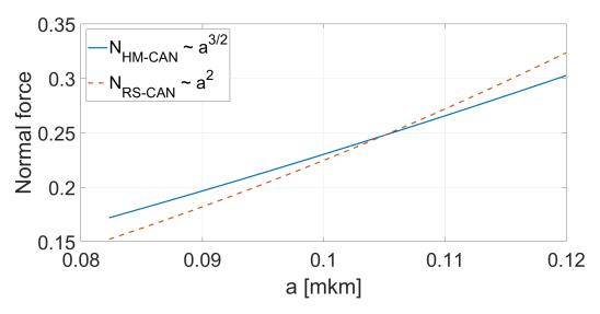
FIGURE 5.10 – The normal load-displacement curve for the HM-CAN and a close curve for RS-CAN with matched parameters for  $m^* = 414$ .
