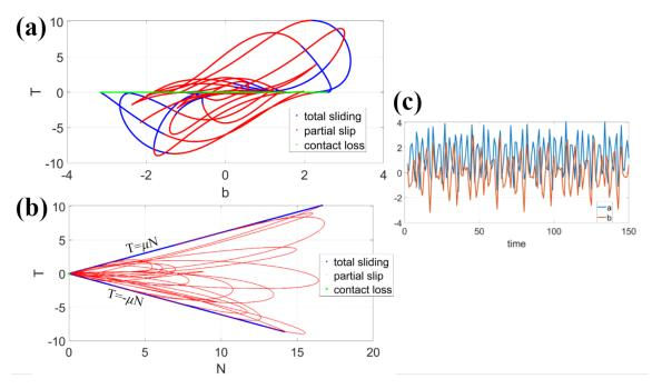
FIGURE 5.7 - (a) Tangential force as a function of tangential displacement and normal force (b) in case of particular displacement histories shown in (c).
