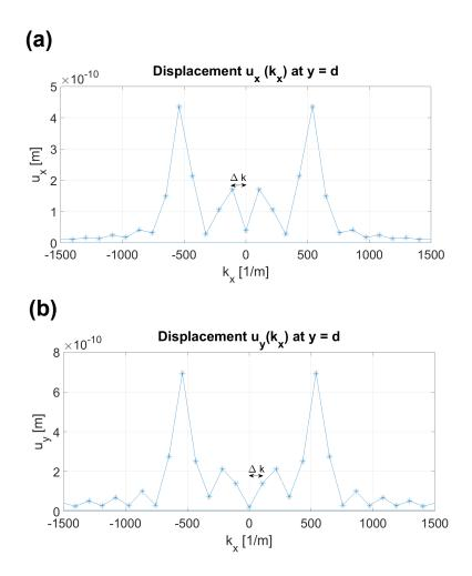
FIGURE 5.18 – Spatial Fourier analysis of secondary waves : displacement (a)  $u_x$  and (b)  $u_y$  as functions of wavenumber  $k_x$  on the top surface of the plate containing the contact acoustic nonlinearity. The dominant component is A0 Lamb wave ( $k_x \approx 540.1 \text{ 1/m}$ ) that the plate was excited with.
