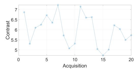
FIGURE 3.8 – Image contrast versus acquisition at different micrometric screw angle. Sphere-plate contact is impregnated with olive oil.
