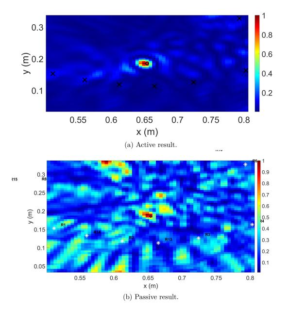
FIGURE 4.8 – Localization results of active vs passive imaging.  $N_s = 18$  emitters and  $N_r = 15$  receivers. The active emitter (0.438, 0.277) m is the same PZT transducer as the one used as a virtual emitter in passive localization. Defect is located at (0.654,0.185) m.
