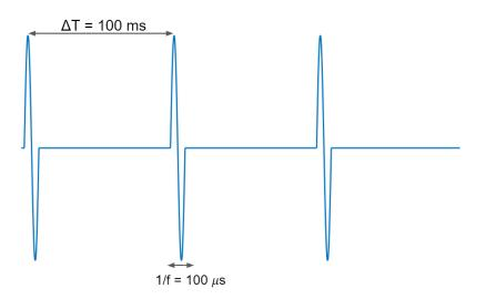
FIGURE 3.3 - Emission signal in static experiments: a sequence of 100 ms one-cycle sine bursts at 10 kHz.
