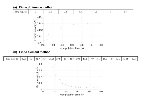
FIGURE 5.15 – Rms error of finite difference (a) and finite elements (b) method comparing to analytical solution for different time meshes as a function of computation time.
