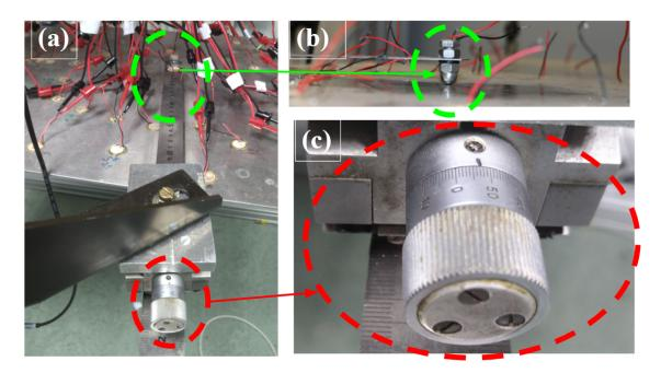
FIGURE 3.4 – Micrometer screw in the defect attaching mechanism allowing to change the angle between the ruler and the plate. (a) - Defect attaching mechanism, (b) - Zoom on the defect, (c) - Zoom on the micrometer screw.
