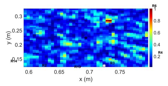
FIGURE 4.5 – Localization result for passive pump-probe experiment  $N_s = 14$  simultaneously emitting uncorrelated noise sources.  $N_r = 14$ . Unsuccessful detection.
