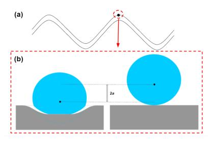
(a) Small ball pressed against a plate is exited by the Lamb wave (plate's deformation is highly exaggerated). (b) Zoom on the ball with the normal contact displacement shown.
