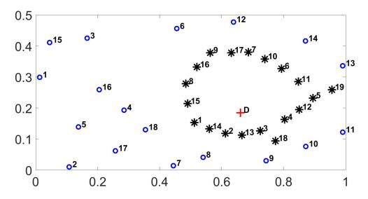
FIGURE 4.7 – Schematic configuration of the considered experiment. The circles denote noise emitters, the asterisks are for receivers and the cross represents defect (CAN) position.
