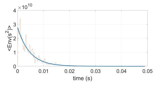
FIGURE 1.5 – Estimation of amplitude A and a plate reverberation time  $\tau$  by using nonlinear least squares fitting for squared signal envelope averaged over receivers.
