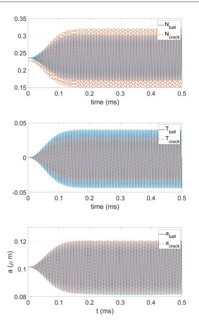
FIGURE 5.11 – Normal (a) and tangential (b) forces applied to the plate by the HM-CAN and RS-CAN with matched normal responses N(a). Here  $m^* = 414$  indicating weak dynamic effects. Frequency f=200 kHz, plate thickness 2d=5 mm, radius of the sphere R=9 mm, no precompression,  $B_{amp} = 0.1$  nm.(c) Normal displacement produced by the HM-CAN and RS-CAN with matched normal responses N(a).
