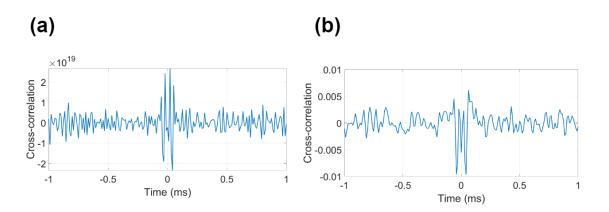
FIGURE 4.4 – Example of cross-correlation function between signals recorded by receivers  $R_1$  and  $R_{14}$  (a) without and (b) with whitening procedure. Cross-correlation of whitened signals are more symmetric with respect to *y*-axis, that implies improved quality of Green's function reconstruction.
