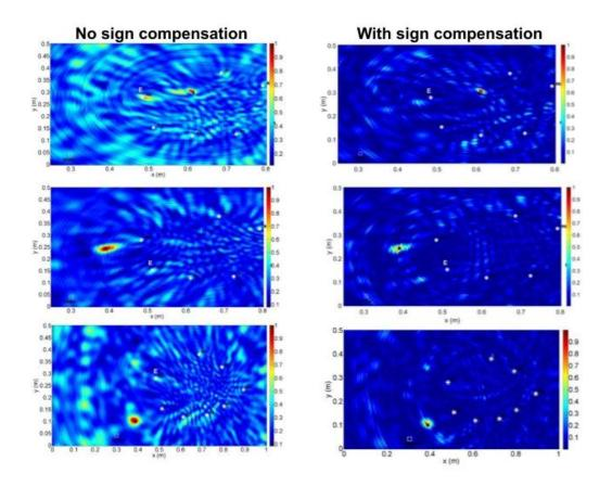
FIGURE 2.12 – Imaging localization results at different defect locations at pump frequency 1.5 Hz : incoherent imaging (left column) and coherent imaging with random sign compensation (right column). White letter E stands for the emitter position : (0.484, 0.278) in top and bottom images, (0.512, 0.153) in the middle ones. White square is for the shaker position (0.3, 0.02).
