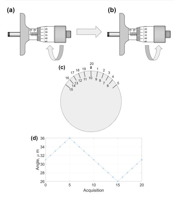
FIGURE 3.5 – Scheme of the experiment with hysteresis : (a) - Turn of a micrometric screw clockwise, (b) - Turn of a micrometric screw counterclockwise, (c) - Schematically shown order of acquisitions (0-20) on the micrometric screw with the distance between two ticks equal 1  $\mu m$ , (d) - Readings on the micrometric screw at different ruler-plate angles as a function of acquisitions.
