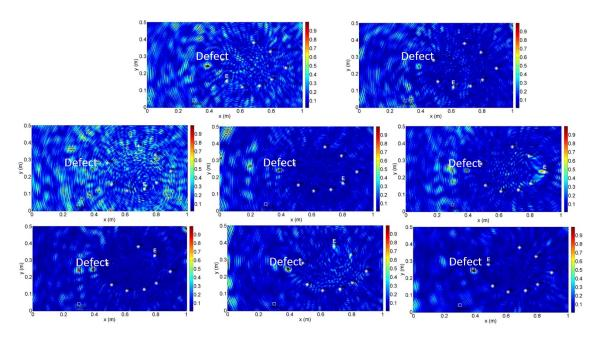
FIGURE 2.10 – Imaging localization results : different PZTs play role of emitter.
