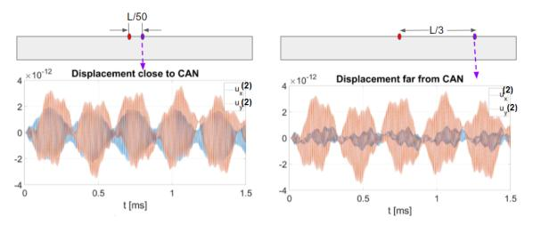
FIGURE 5.17 – Secondary waves emitted by Hertz-Mindlin CAN in a thin plate.
