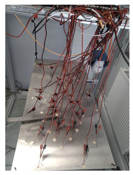
FIGURE 4.1 – Passive experimental setup with multiple simultaneous noise sources.
