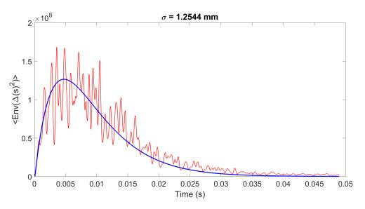
FIGURE 1.6 – Estimation of a parameter K by using nonlinear least squares fitting for squared differential signal envelope averaged over receivers.
