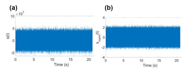
FIGURE 4.2 – Recorded signal : (a) before and (b) after the normalization in time.
