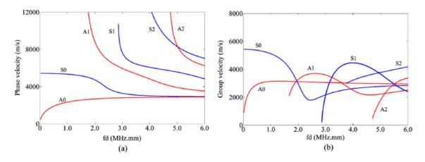
FIGURE 1.2 – (taken from Liu et al. [15]) Dispersion curves of Lamb waves in an aluminum plate : (a) phase velocity and (b) group velocity.
