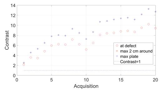
(b) Comparison between different definitions of contrast versus number of acquisitions in pump-probe experiment.
