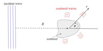
FIGURE 1.4 – Wave scattering by a rigid heterogeneity.
