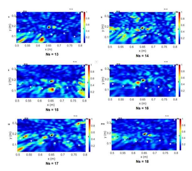
FIGURE 4.13 – Localization images with different number of noise sources  $N_s$ .
