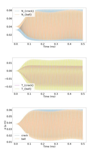
FIGURE 5.12 – Normal (a) and tangential (b) forces applied to the plate by the HM-CAN and RS-CAN with matched normal responses N(a). Here  $m^* = 155$  that corresponds to moderate dynamic effects. Frequency f=200 kHz, plate thickness 2d=3 mm, radius of the sphere R=5 mm, no precompression,  $B_{amp} = 0.15$  nm. This HM-CAN mimics real damage only qualitatively.(c) Normal displacement produced by the HM-CAN and RS-CAN with matched normal responses N(a).
