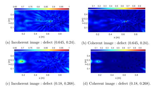
FIGURE 2.9 – Localization results for synchronized experiments with incoherent imaging (left column) and coherent imaging with synchronous detection (right column).
