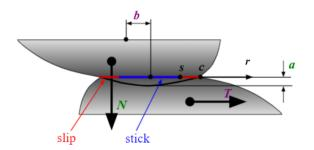
FIGURE 5.3 – Illustration of the partial slip regime for an example of two spheres pressed against each other. Blue segment denotes stick zone, red segments are for slip zone.
