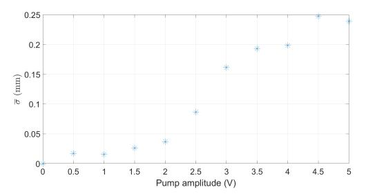
FIGURE 3.13 – Scattering cross-section against pump amplitude in active dynamic experiment.
