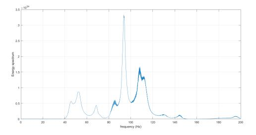
FIGURE 2.8 – Energy spectrum of the plate.
