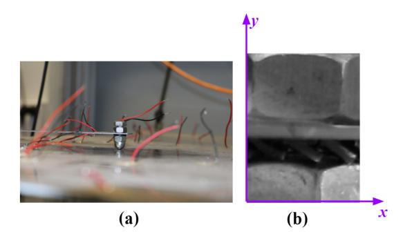
FIGURE 2.3 – (a) - Frame of a video of the pump-probe experiment : zoom on the defect, (b) - gray scale fragment of this frame selected for image correlation procedure to estimate the sphere's y-displacement induced by pump excitation.
