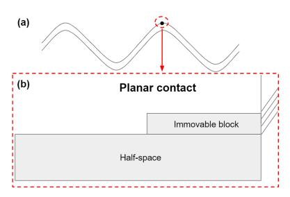
(a) Two rough surfaces in contact exited by the Lamb wave (plate's deformation is highly exaggerated). (b) Zoom on the RS-CAN.
