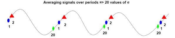
FIGURE 3.11 – Averaging signals over periods for scattering cross-section measurement in pump-probe experiments.
