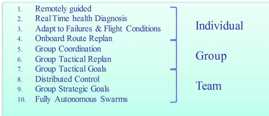
Fig. 16 Autonomous Control Levels (Adapted from the Roadmap proposed by the Department of Defense of the United States to design Unmanned Aerial vehicles (Galster et al., 2007))
