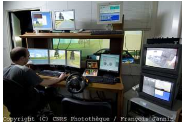
Fig. 47 Control room of UPHF's car driving simulator
