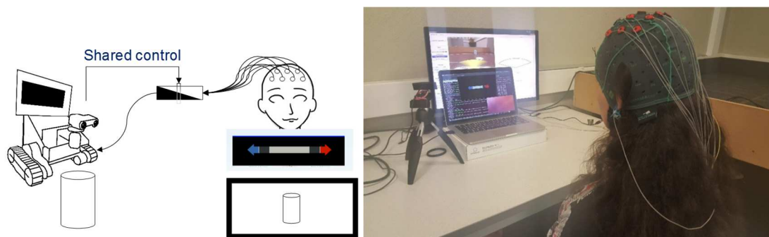
Fig. 79 Human-BCI-robot cooperation - Shared control with “emulated haptic feedback”
