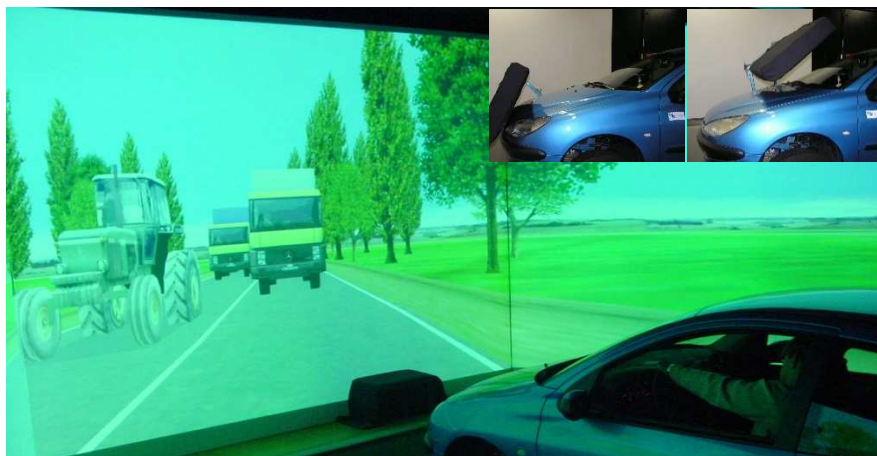
Fig. 72 Scenario of the unavoidable crash situation; Sequence of the falling block on the windscreen
