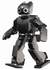
FIGURE 1.22 – Le robot humanoïde Darwin-OP (Dynamic Anthropomorphic Robot with Intelligence Open Platform).
