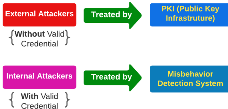
Figure 2.6: Type of Attacker in Vehicular Network
